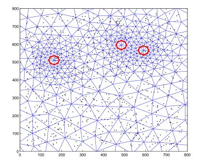
Figure 8. Random scenario with 3 heat sources and 1000 sensor nodes.
