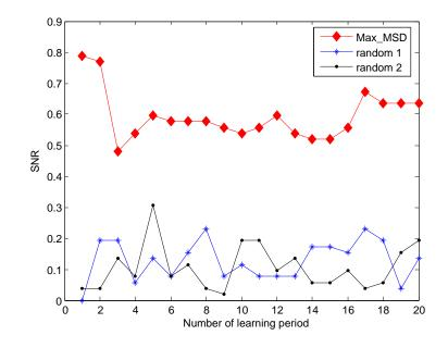
Figure 5. Effect of active nodes selection using the  $Max_MSD$  and *random* approaches on SNR.
