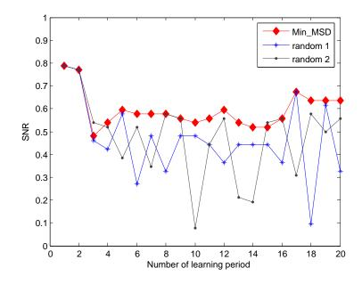
Figure 4. Effect of cluster head selection using the  $Min_MSD$  and random approaches on SNR.
