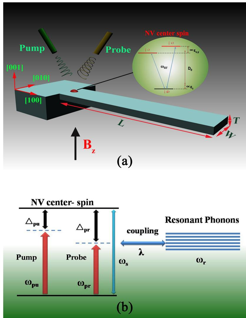
**Figure 1.** (a) Schematic diagram of the hybrid spin-microcantilever system in the presence of a strong pump field and a weak probe field. The inset is the energy level diagram of a nitrogen vacancy (NV) center spin.  $[\varepsilon_i]_{i=x,y,z}$  are the diagonal components of the strain tensor defined in the NV's basis (note that we have neglected shear); (b) The energy level diagram of the coupling between the NV center spin and the microcantilever.
