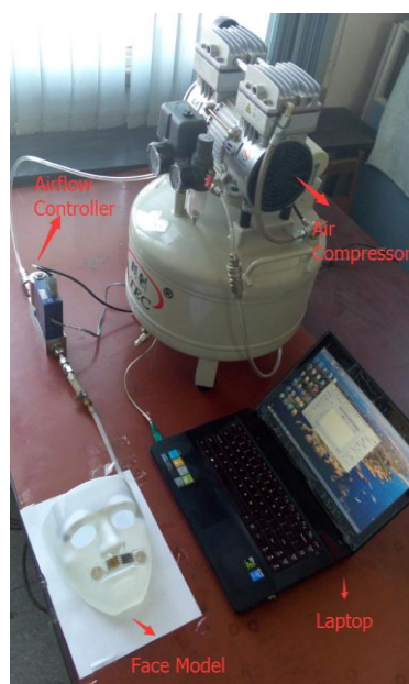
Figure 11. Experimental setup for respiration simulation.
