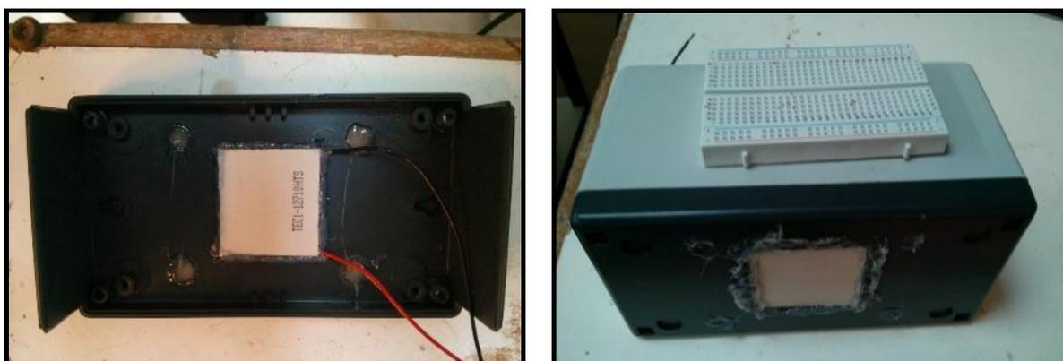
**Figure 9.** Peltier cell installation.
