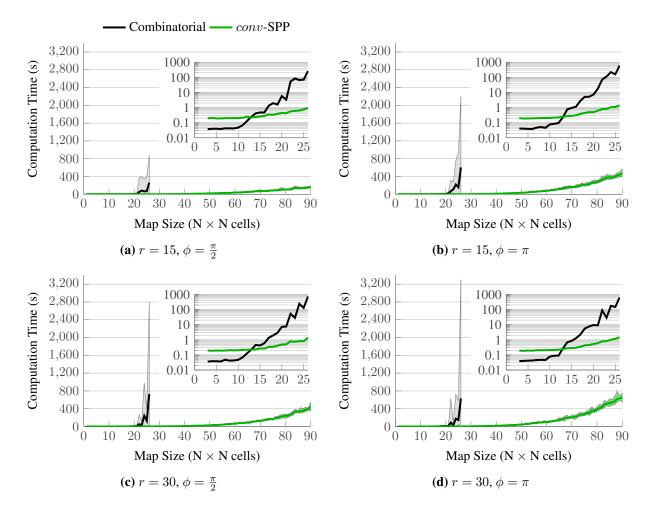
**Figure 13.** Computation times to calculate the optimal solutions and to solve the instances with *conv*-SPP. The thick lines represent the average computation times for each set of maps, while the colored intervals are bounded by the minimum and maximum times it took to solve all the instances in one set. The inset graphs show the computation times on a logarithmic scale.
