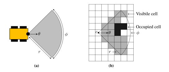
**Figure 3.** (a) a candidate sensing configuration c allows the robot to scan a circular sector of central angle  $\phi$  and radius r; (b)  $v_{\mathcal{P}}(c)$  is the visibility function which defines which are the cell that are observable from candidate sensing configuration c.
