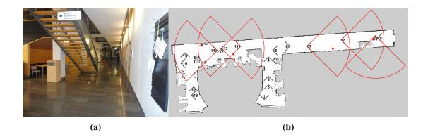
**Figure 15.** (**a**) an indoor setting for the gas detection task; (**b**) graphical results: the gas sources are indicated by red dots, the planned sensing configuration by truncated cones in gray, and the small number associated to each configuration indicates the order in which they are visited. The configurations plotted in red indicate the positive readings and the actual area they cover.
