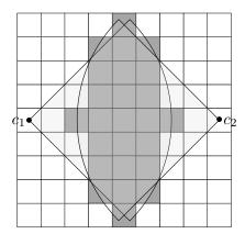
Figure 10. The sensing configurations  $c_1$  and  $c_2$  are trapped in a local minimum. The cells under the overlapping field of view are indicated in gray. Assuming that the remaining visible cells of both configurations, indicated in white under the coverage window, are partially (50%) observed by another configuration(s) in the solution. The  $c_1$  and  $c_2$  are set to 0.5 in the solution vector and any subsequent iteration does not improve the situation.
