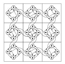
**Figure 2.** The graph captures the allowed movements of the robot on a grid map when  $\Theta = \{0, \frac{\pi}{2}, \pi, \frac{3}{2}\pi\}$  and only forward movements are allowed. Small circles indicate the poses where the robot can stop (the internal arrow indicates the orientation of the robot) and the directed edges its allowed movements. Note that in the figure the poses do not correspond to the centers of the cells, but this is only for clarity reasons.
