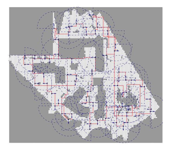
**Figure 14.** The exploration plan generated for the map of the Freiburg University campus (obstacles are represented in gray). The positions of the sensing configurations are represented with blue dots, blue arrows indicate their orientation and dashed-lines their field of view. A closed path through the configurations is shown in red.
