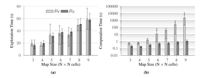
**Figure 7.** Comparison of two disjoint approaches up to maps of size  $9 \times 9$ . Notations are similar as in the previous figure, *i.e.*, bars indicate the average values over the 3 maps for  $3 \times 3$  and 10 maps for the rest, and error bars indicate the minimum and maximum values observed during the trial. (**a**) shows the solution quality of two disjoint approaches  $(D_T, D_S)$ ; and (**b**) shows the average computation time on a logarithmic scale for both approaches.
