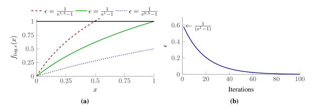
Figure 9. (a) Smaller value of  $\epsilon$  defines steeper penalty functions; (b) The exponential decay of  $\epsilon$  during the iterative procedure.
