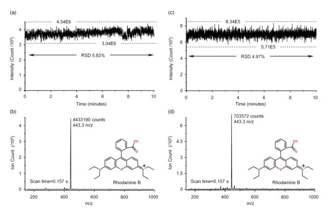
**Figure 6.** Data acquired while infusing 10  $\mu$ M Rhodamine B in 50/50 (v/v) methanol/water containing 0.2% acetic acid at an injection pressure of 25 mbar. The electrospray potential was +4.5 kV. (**a**,**c**) Rhodamine B ion counts and signal stability of the proposed corner integrated emitter and the fused-silica capillary, respectively; (**b**,**d**) Single spectra over a 0.157 seconds scan time of the proposed corner integrated emitter and the fused-silica capillary, respectively.
