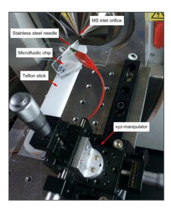
**Figure 3.** Experiment platform. A laboratory-built platform was set up on the commercial ion trap MS to perform the microchip experiments.
