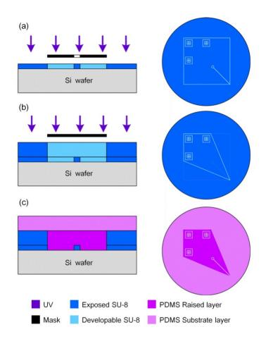
**Figure 2.** Process schematic. (a) the first *ca*. 30  $\mu$ m thick SU-8 photoresist layer was subjected to UV exposure; (b) the second *ca*. 180  $\mu$ m photoresist layer was subjected to UV exposure with another mask; (c) PDMS pre-polymer was poured onto the photoresist master and the raised and substrate layers were both formed.
