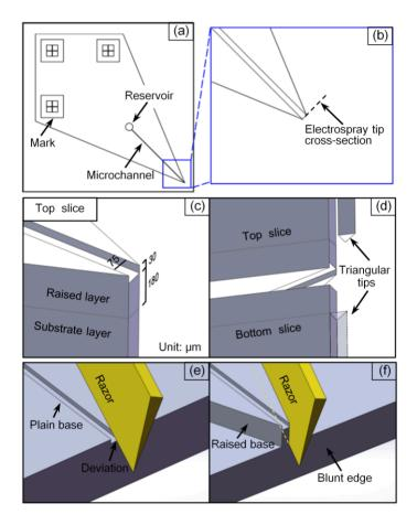
Figure 1. Diagrams of the chip's design and fabrication. (a) AutoCAD design of the microfluidic emitter-integrated chip;  $(\mathbf{b},\mathbf{d})$  blunt configuration for the chip corner tip emitter, eliminating the influence of triangular tips in top and bottom slices; (c) dimensions of the top slice;  $(\mathbf{e},\mathbf{f})$  comparison between plain and raised bases for chip cutting: there will be deviations arising from the use of a plain base.
