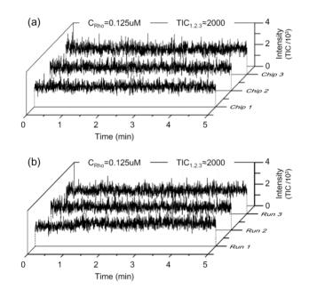
**Figure 8.** Reproducibility of chip-to-chip and run-to-run tests. (a) The mean ion counts of Rhodamine B were 1969.90, 2137.60 and 2055.85 for chips 1 to 3, respectively when the solution concentration was 0.125  $\mu$ M; (b) the mean ion counts were also approximately 2000 for run 1 to 3 of chip 2. The solution concentration was 0.125  $\mu$ M.
