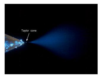
**Figure 5.** Image of the laser-illuminated electrospray: this is a frame captured from video footage of the electrospray plume generated from the corner integrated emitter tip.
