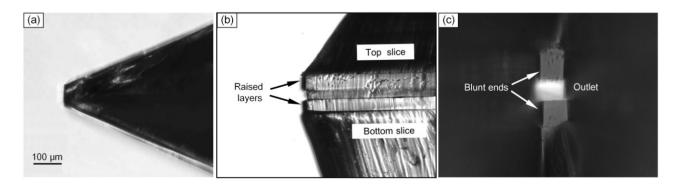
**Figure 4.** Micrographs of the corner integrated emitter. (a) Top view of the *c*. 75  $\mu$ m blunt tip of the 45° corner; (b) Lateral view of the tip, the micro-channel layer lies between the two raised layers; (c) Front view of the tip: the blunt ends and outlet are clearly distinguishable.
