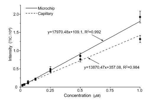
**Figure 7.** Different signal intensities of sample solutions in different concentrations. Each point represents the mean value of signal data and error bar for the deviation at each concentration.
