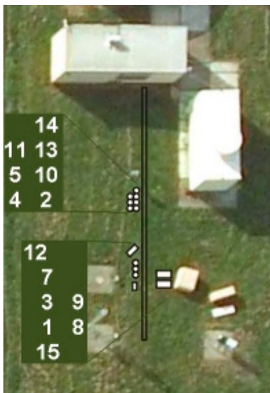
**Figure 3.** Top view of the CLIC instrument setup of the SQMs. Locations are indicated by white circles and rectangles. Insets show the corresponding numbers. As SQM 6 arrived late on the site and did not join the official CLIC-campaign period, it was placed at location 11 after the campaign.
