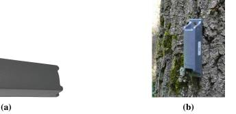
**Figure 8.** Sensor node package hosting the PCB, a half-AA battery and the normal mode helix antenna (NMHA) antenna. The aperture on the left improves the NTC thermal contact (**a**); fixed on trees with screws (**b**).
