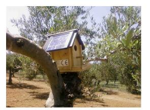
(b) Gateway 2 is deployed in the field high above the ground to improve its RF coverage. The ground of the test field is clean, facilitating navigation and sensor deployment and retrieval.
