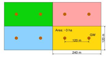
**Figure 5.** The network is made of independent cells with a star topology inside (the distances assume a 200 m sensor communication range). The sensors in each cell are covered by two gateways, which can independently contact the server to ensure redundant field message aggregation and upload. Larger areas can be covered by joining elementary cells.
