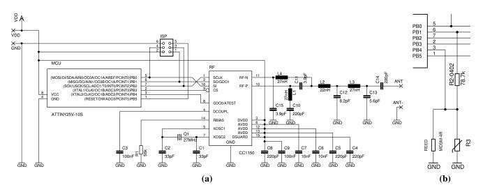
Figure 7. Schematic of the sensor node prototype for laboratory testing (**a**); issues fixed (**b**): (1) add a temperature transducer with an interface circuit and (2) add a means to switch the sensor to deployment mode.
