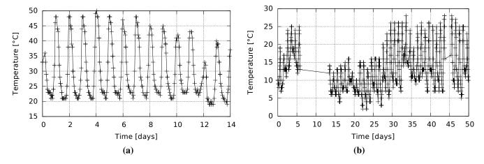
**Figure 12.** Gateway temperature can exceed  $45 \,^{\circ}$ C, the maximum allowed for lithium-ion battery charging (**a**), while the internaloscillator drift can break the synchronous serial communication with the GPRS modem at low temperatures (Days 6–13 and 43–45) (**b**).
