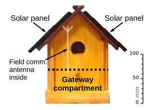
(a) The birdhouse has solar panels on the roof and the gateway, battery and GPRSmodem in a sealed package at the bottom. The antenna between the solar panels has low RF performance.
