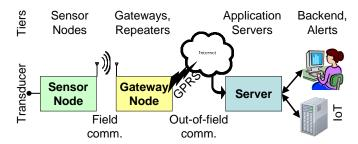
Figure 1. Typical tiered structure of WSN platforms.
