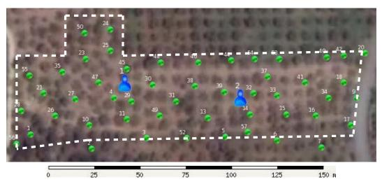
**Figure 6.** The test field is about is about  $195 \times 45$  m (main body). Trees appear as darker spots on the light-colored soil. There are two gateways and 50 sensor nodes (round dots; some are placed outside the field due to GPS positioning errors).
