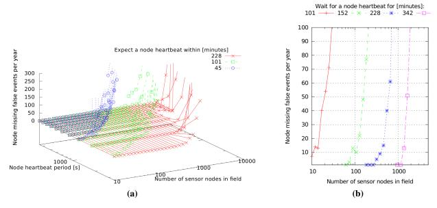
**Figure 2.** Simulation results of the field communication protocol for design space exploration. The rate of the missing node erroneous reports increases with the number of nodes and with the heartbeat period and lowers with the increase of the heartbeat listening window of the gateway ( $\mathbf{a}$ ); missing nodes can be detected in less than 6 h with a negligible rate of erroneous reports, for a 1 h heartbeat period ( $\mathbf{b}$ ).
