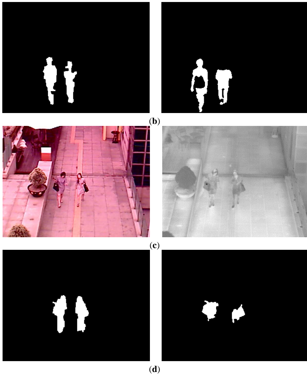
Figure 5. Examples obtained from CWI. (a) First example of the current input images by visible light (left figure) and thermal cameras (right figure) in morning; (b) Detected CWIs in visible light (left figure) and the thermal input image (right figure) of (a); (c) Second example of the current input images by visible light (left figure) and thermal cameras (right figure) at afternoon; (d) Detected CWIs in visible light (left figure) and the thermal input image (right figure) of (c).
