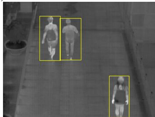
Figure 9. Examples of combined image of CWI and CSI, and the final result of human detection. (a) Combined image of CWI (right image of Figure 7b) and CSI (Figure 7c); (b) Final result of human detection.
