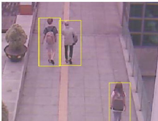
Figure 9. Examples of combined image of CWI and CSI, and the final result of human detection. (a) Combined image of CWI (right image of Figure 7b) and CSI (Figure 7c); (b) Final result of human detection.
