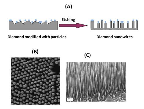
**Figure 4.** (A) Top-down etching process of CVD diamond using seed particles; (B) SEM image of diamond cylinders obtained using oxygen reactive ion etching (RIE) for 60 min through a 1  $\mu$ M SiO<sub>2</sub> particle array (reprint with permission from [18]); (C) SEM image of vertically aligned diamond nanowires using diamond nanoparticles as masks (with courtesy of C. Nebel).
