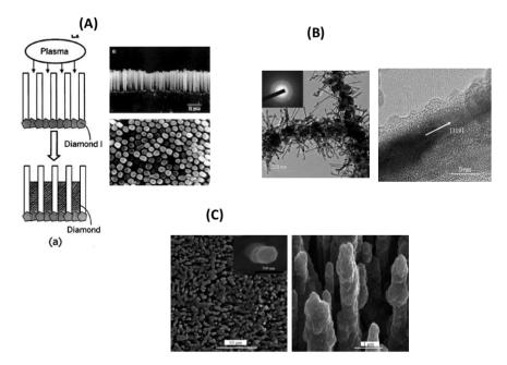
Figure 6. (A) Schematic diagram of the bottom-up fabrication of cylindrical diamond wires in porous alumina template (left) and the corresponding SEM images (reprint with permission from [28]); (B) TEM (left) and HR-TEM (right) images of diamond rods grown on carbon nanotubes (reprint with permission from [29]); (C) SEM image of diamond coated silicon nanowires (reprint with permission from [10]).
