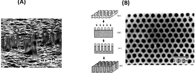
Figure 3. (A) SEM images of diamond nanowiskers formed on as-grown diamond films coated with 400 nm thick Al layer using reactive ion etching (RIE) with oxygen plasma (reprint with permission from [16]); (B) Formation of honeycomb diamond films (reprint with permission from [15]).
