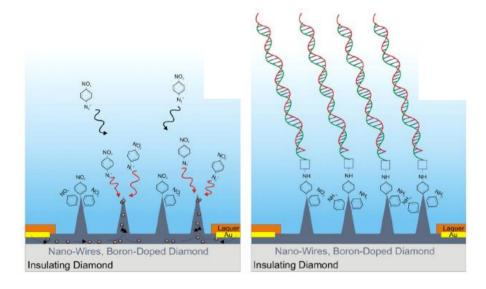
**Figure 8.** Diamond nanowires for DNA sensing: Preferential linking of phenyl aryl and DNA molecules to the tip of the wires (reprint with permission from [23,44]).
