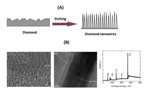
**Figure 5.** (**A**) Top-down etching process of CVD diamond without mask; (**B**) SEM and HR-TEM images, and XPS survey spectrum of boron-doped diamond nanowires synthesized through maskless technique (reprint with permission from [26]).
