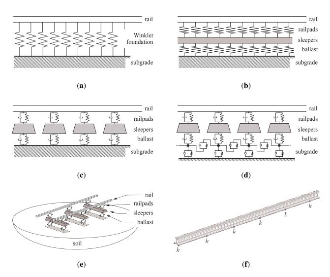
Figure 8. Track modelling: a review. (a) 2D single layer track model (continuously supported); (b) 2D two layer track model (continuously supported); (c) 2D two layer track model (discretely supported); (d) 2D three layer track model (discretely supported); (e) 3D three layer track/soil model (discretely supported); (f) 3D model for the rail (discretely supported).
