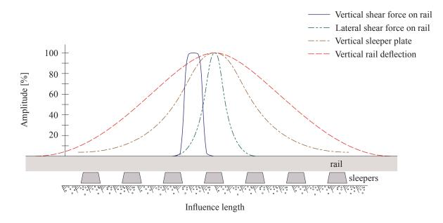
Figure 10. Qualitative influence of load measurement on track (adapted from [40]).
