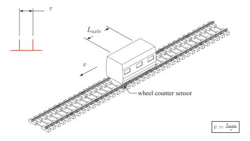
Figure 1. Speed evaluation based on wheel counters.
