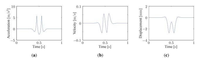
Figure 12. Track deflection due to the passing of a single bogie. (a) Acceleration;(b) Velocity; (c) Displacement.
