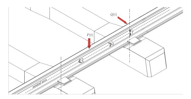
Figure 11. Wheel/rail vertical and lateral forces estimation using strain gage circuits.
