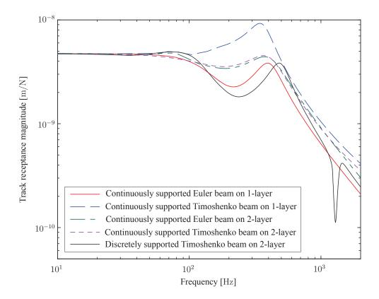
Figure 9. Track receptances calculated using numerical codes.
