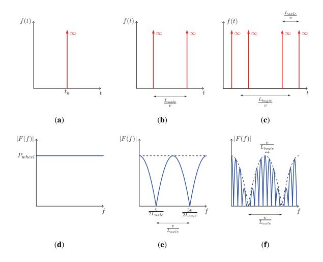
Figure 4. Carbody effect with Dirac functions. (a) Single Dirac function—one wheel effect (time history); (b) Double Dirac function—two wheels effect (time history); (c) Quadruple Dirac function—four wheel effects (time history); (d) Single Dirac function—one wheel effect (frequency content); (e) Double Dirac function—two wheels effect (frequency content); (f) Quadruple Dirac function—four wheel effects (frequency content).
