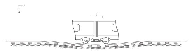
Figure 7. Track deflection generated by the passing of a train.
