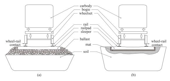
Figure 3. Vehicle/track main components (longitudinal view). (a) Ballasted track;(b) Slab track.
