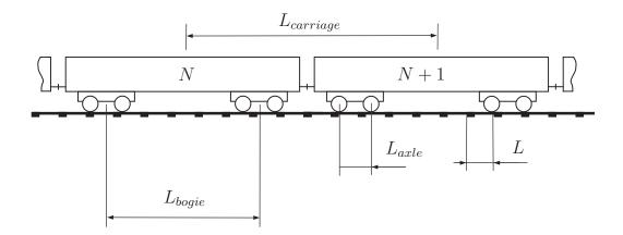
Figure 5. Rudimentary geometrical parameters of the train and the track ([17]).
