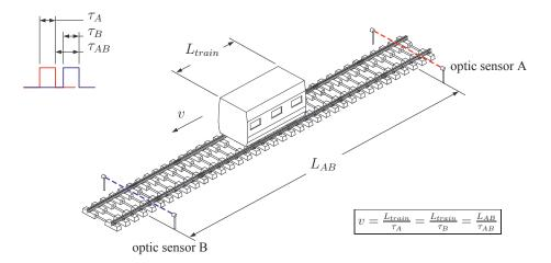
Figure 2. Speed evaluation based on two optic sensors placed along the track.
