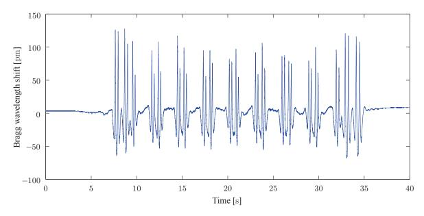
Figure 13. Trace (Bragg wavelength shift with time) of an FBG glued on the foot of a 50E2 rail and subject to a train circulating at 40 km/h.
