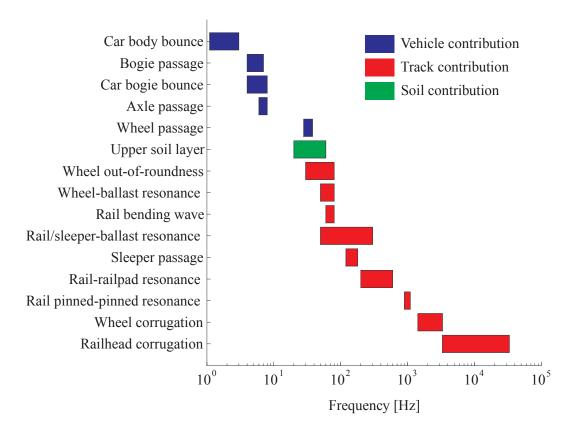
**Figure 6.** Main contribution of dynamic vehicle/track and soil interactions (with permission from [21]).
