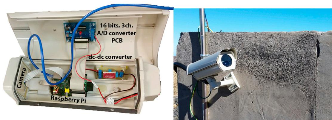
**Figure 16.** Imaging monitoring system.
