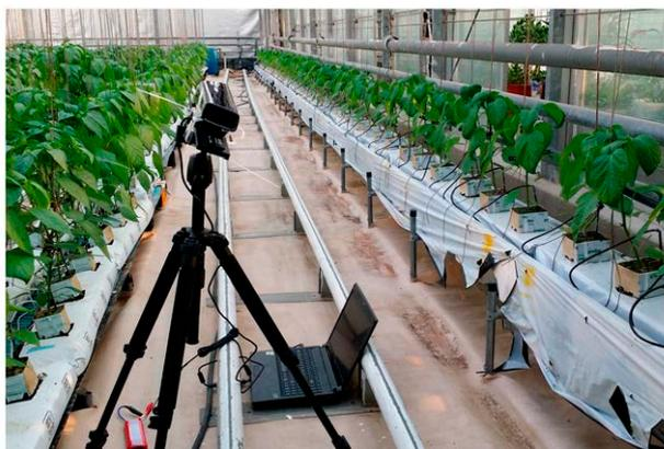
**Figure 1.** Structure of plant monitoring using Kinect camera in the green house.
