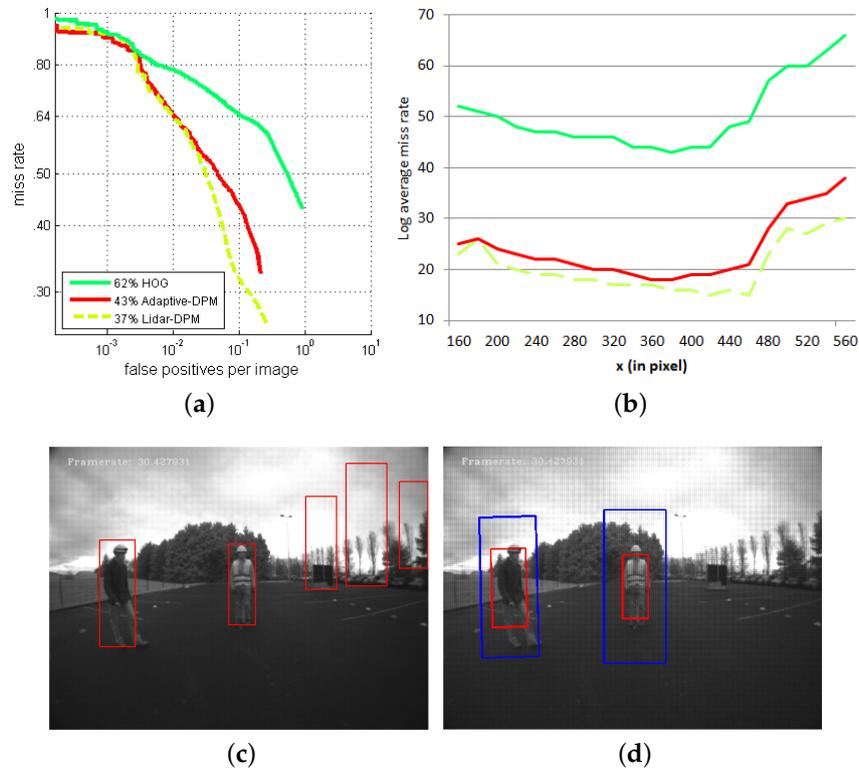
**Figure 17.** Comparison of detection performance between the exclusively vision-based approaches and the LiDAR-fisheye camera PDS in Configuration 1: (a) ROC curve, (b) miss rate for lateral image position, (c) vision-only detections and (d) LiDAR-fisheye detections.
