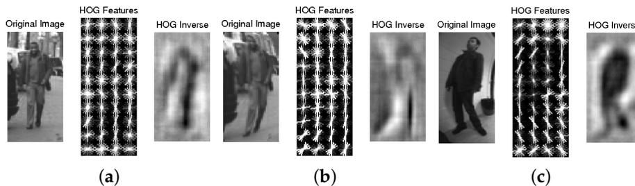
**Figure 11.** HOG features visualization in artificial distorted image samples. (a,b) The original  $48 \times 96$  training sample image and its distorted version; (c) original distorted image sample captured by a fisheye camera.
