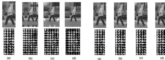
**Figure 7.** Visualization of HOG features from different border extension methods before (left part) and after (right part) the distortion process: (a) original image; (b) mirror extension; (c) mirror-inverted extension; (d) duplicate extension.
