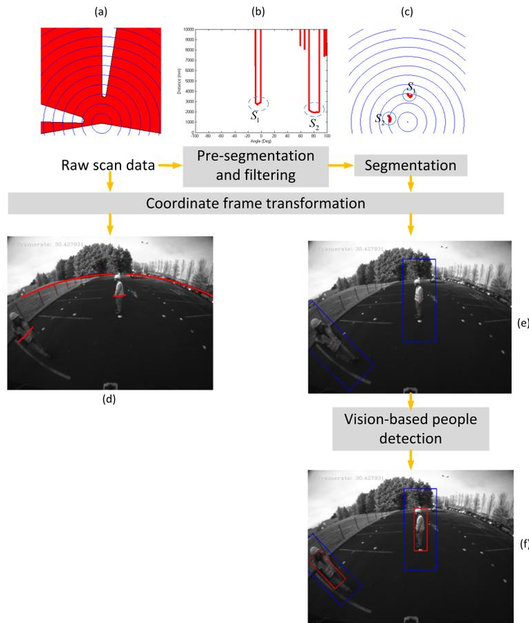
**Figure 15.** Processing steps in the LiDAR-based pedestrian detection system (PDS). (a) LiDAR points in polar coordinates; (b) point distance filtering; (c) two segments correspond to two obstacles in the FOV; (d) projection of points using calibration information; (e) image projection of adaptive ROIs; (f) final result of LiDAR-based PDS.
