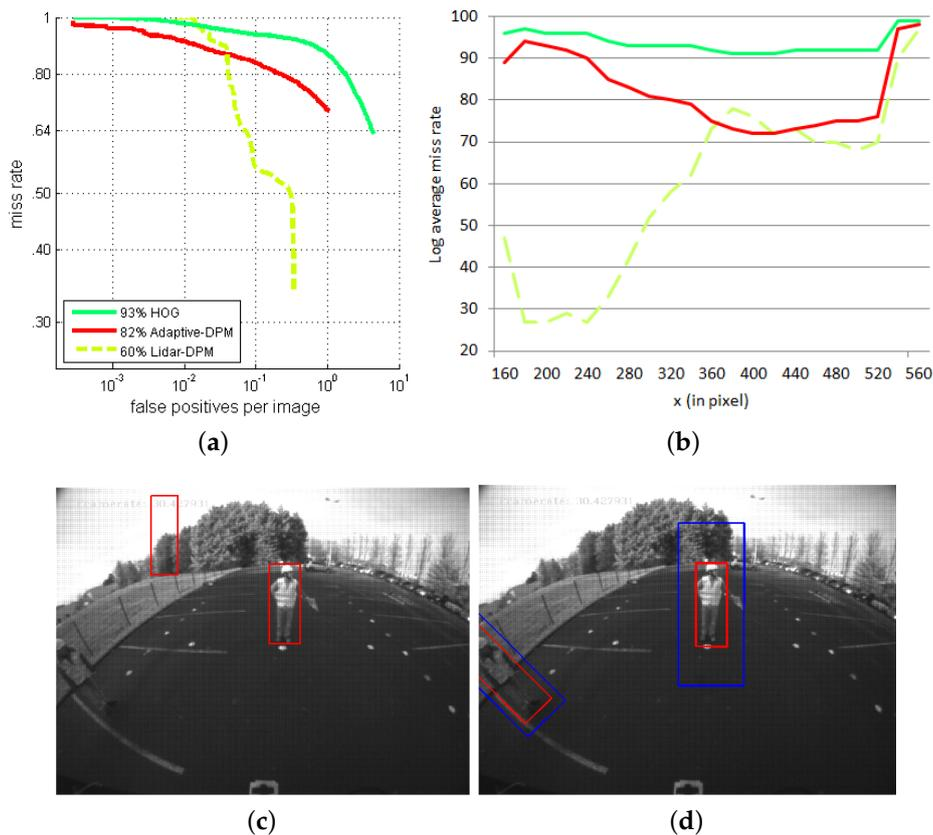
**Figure 18.** Comparison of detection performance between the exclusively vision-based approaches and the LiDAR-fisheye camera PDS in Configuration 2: (a) ROC curve, (b) Miss rate for lateral image position, (c) vision-only detections and (d) LiDAR-fisheye detections.
