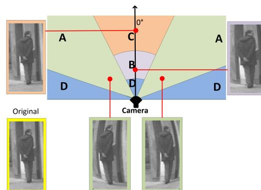
**Figure 5.** Artificial distorted images and their corresponding positions on the fisheye camera's FOV. The sample image are simulated at  $-45^\circ$ ,  $0^\circ$  and  $45^\circ$  at a distance of 1.2 m.
