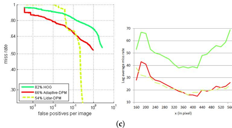
**Figure 20.** Comparison of detection performance between the exclusively vision-based approaches and the LiDAR-fisheye camera PDS in different machine operating states: (a) static, (b) turning and (c) forward.
