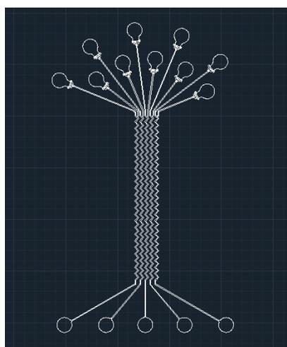
**Figure S2.** Channel geometry of the polydimethylsiloxane (PDMS) microfluidic device. The microchannel height is 40  $\mu\text{m}$  and width is 100  $\mu\text{m}$ .
