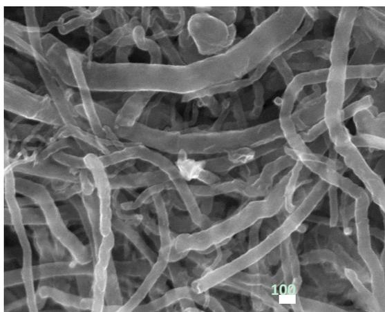
**Figure S1.** Scanning electron microscopy (SEM) image of pristine multi-walled nanotubes (MWNTs).
