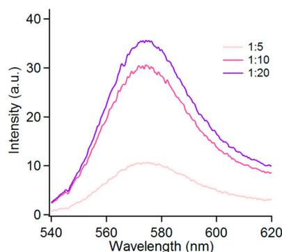
**Figure S3.** Fluorescence spectra of P1 (100 nM) in the presence of different ratios of MoS<sub>2</sub>/MWCNT (1:5, 1:10, and 1:20). The concentrations of the different MoS<sub>2</sub>/MWCNT ratios are all 150 µg/mL.
