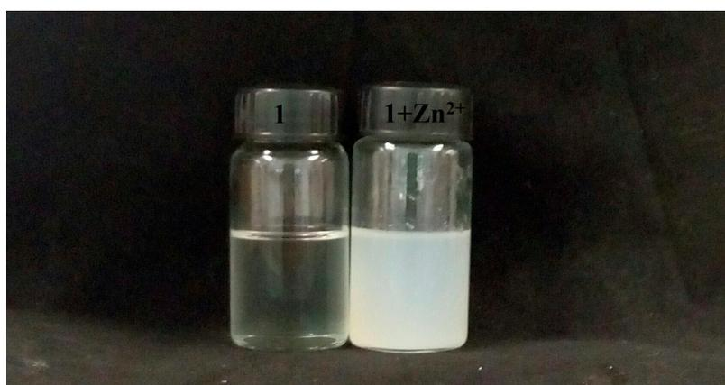
**Figure S9.** Images of **1** at high concentration in DMSO-H<sub>2</sub>O (1/1, *v/v*) before and after the addition of Zn<sup>2+</sup> under daylight.
