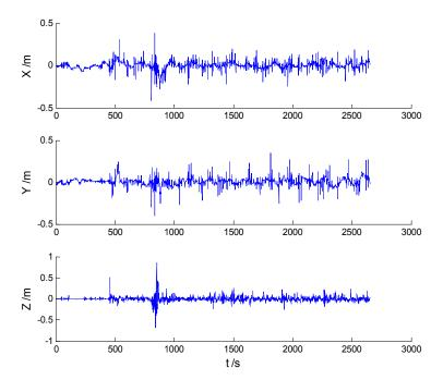
Figure 2. Position errors of the Kalman filter (KF) algorithm.
