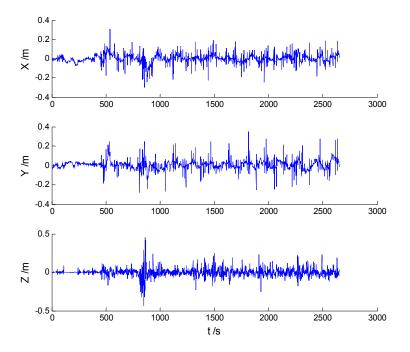
Figure 3. Position errors of the adaptive Kalman filter (AKF) algorithm.
