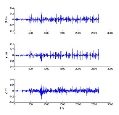
Figure 5. Position errors of the adaptive H-infinity filter (AHF) algorithm.
