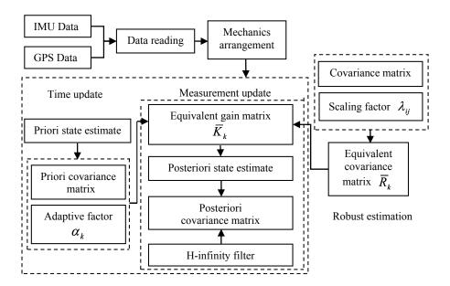
Figure 1. A flow chart of the adaptive H-infinity algorithm.
