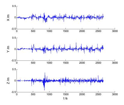
Figure 4. Position errors of the H-infinity filter (HF) algorithm.
