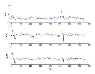
Figure 6. Position errors of the KF algorithm.
