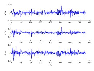
Figure 9. Position errors of the AHF algorithm.
