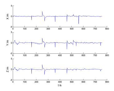
Figure 11. Position errors of the AKF algorithm.
