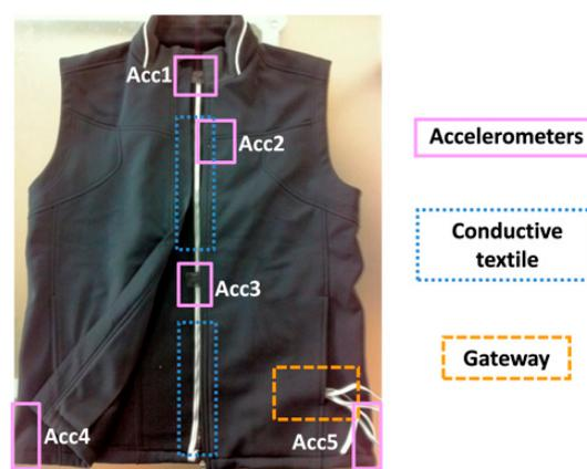
Figure 3. The fully developed wearable instrumented vest.
