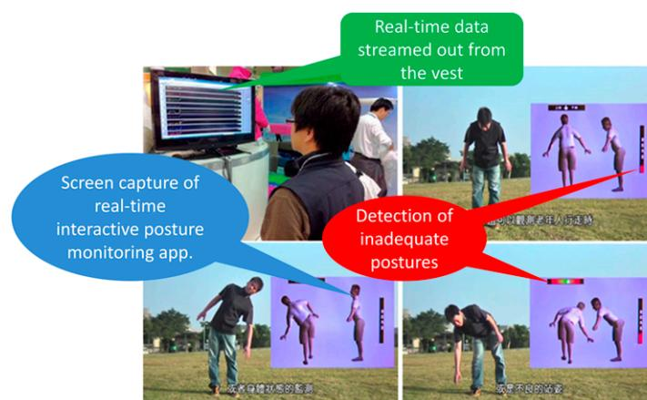
**Figure 4.** Interactive posture monitoring and real-time warning application.
