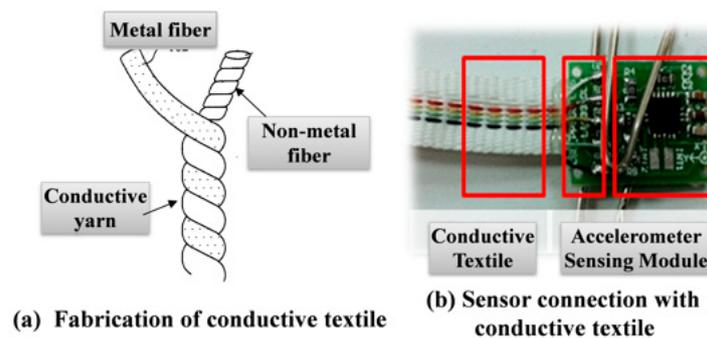
**Figure 2.** Conductive textile: (a) fabrication schematics; and (b) integrated with sensing module.
