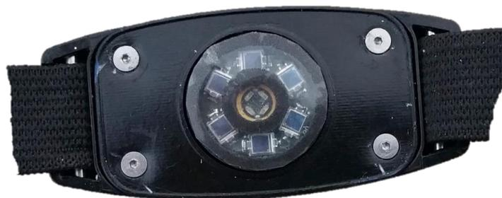
**Figure 1.** Six-photodetector (6PD) Forehead Mounted Reflectance-Mode Multichannel Photoplethysmographic (MCP) Sensor.
