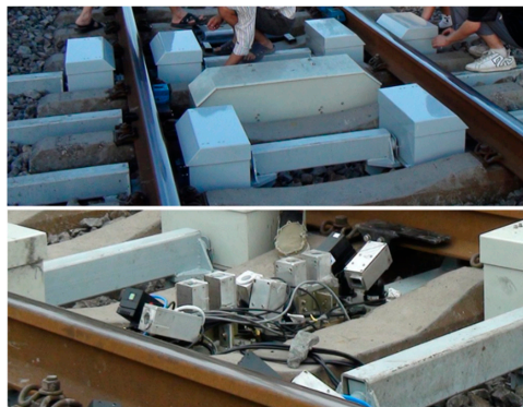
Figure 21. Wheelset dynamic measurement system installed on the railway bed.
