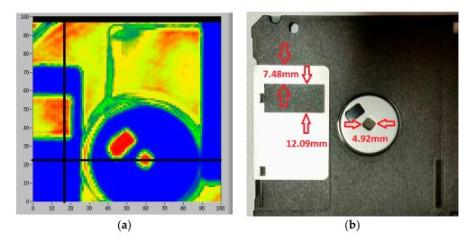
**Figure 4.** (a) A transmission image of a computer floppy disk; a scanned area of 50 mm  $\times$  50 mm at a resolution of 0.5 mm. The black lines indicate the single line scans at vertical line 17 and horizontal line 23; (b) is the photograph of the floppy disk flipped to correspond to scanned image.
