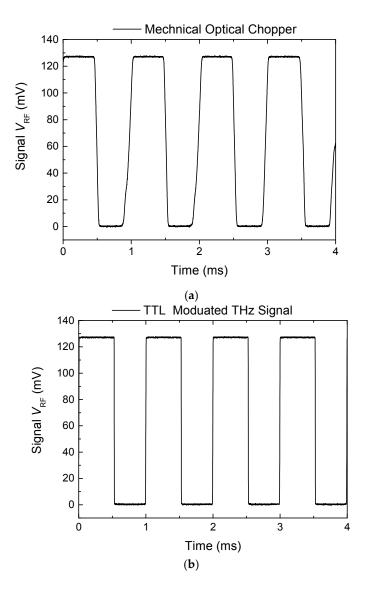
**Figure 9.** Real-time detector voltage output  $V_{RF}$  (t) traces of the modulated THz beam using a mechanical optical chopper (**a**) and an electronic signal via the TTL port on the AMC THz source (**b**).
