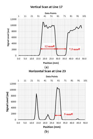
**Figure 5.** Line scans of the image data: the detected signal level of the transmitted THz beam *versus* the pixel point (upper *x*-axis) and spatial position (lower *x*-axis). (a) corresponds to the single line scans at vertical line 17 in Figure 4a and (b) corresponds to the horizontal line 23 shown in Figure 4a. The upper *x* axis shows the image pixel points (0.5 mm each step) and lower axis is converted the position points in both figures.
