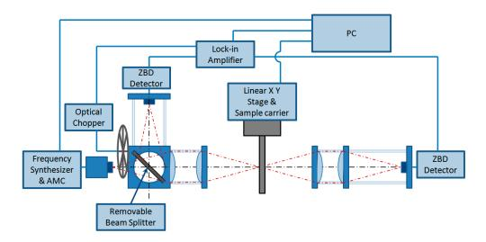
Figure 3. Schematic of the quasi-optical THz transmission and reflection imaging system.
