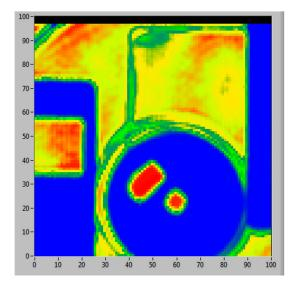
**Figure 10.** The THz transmission image of the computer disk acquired using the TTL electronic signal modulation at the same chopper speed of 1 kHz and scanning conditions as that used in Figure 4 image modulated with an optic chopper.
