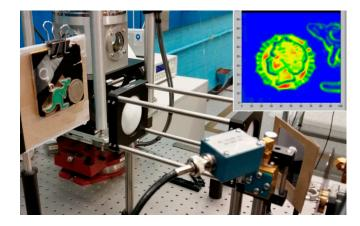
**Figure 6.** Imaging of a 50 cents coin and a Kangaroo key ring in a reflection mode (note that the experiment was carried out before the introduction of the cube mounted beam splitter shown in Figure 2).
