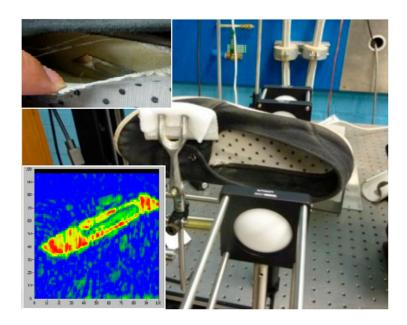
Figure 7. Imaging in reflection mode, showing a hidden object in shoe lining.
