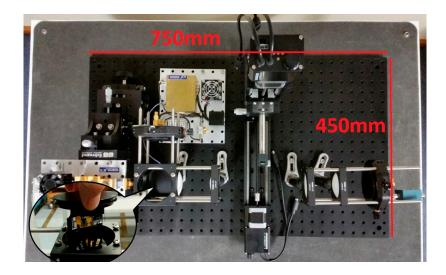
**Figure 2.** A view of the full system mounted on a portable optical plate ( $450 \text{ mm} \times 750 \text{ mm}$ ) showing a linearly aligned source-lenses-sample-detector scheme and a removable beam splitter (inset) for changing between transmission and reflection mode.
