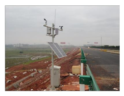
Figure 4. Small weather station (site picture).
