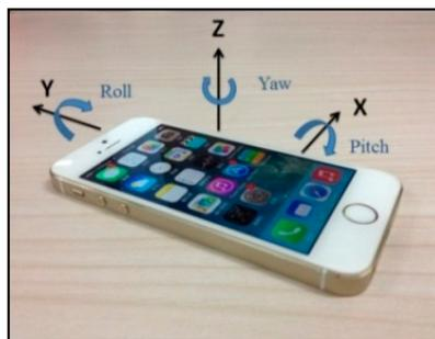
Figure 4. Angle-of-rotation directions.
