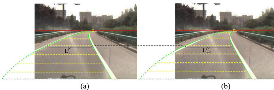
**Figure 8.** Shape similarity of lane boundaries in two consecutive frames. (a) Lane boundary detection in the  $n$ -th frame; (b) Lane boundary detection in the  $(n + 1)$ -th frame.
