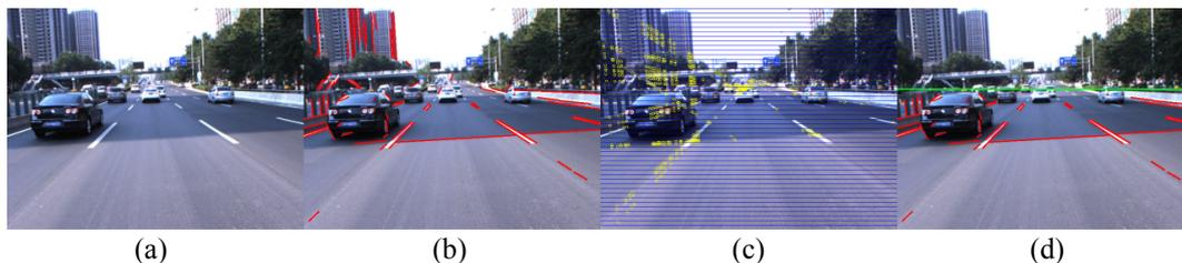
**Figure 2.** Feature extraction. (a) Original image; (b) Line Segment Detector (LSD) result; (c) Horizontal bands in the image; the yellow points represent the crossing points of line segments; (d) Line segments above the vanishing line are eliminated.
