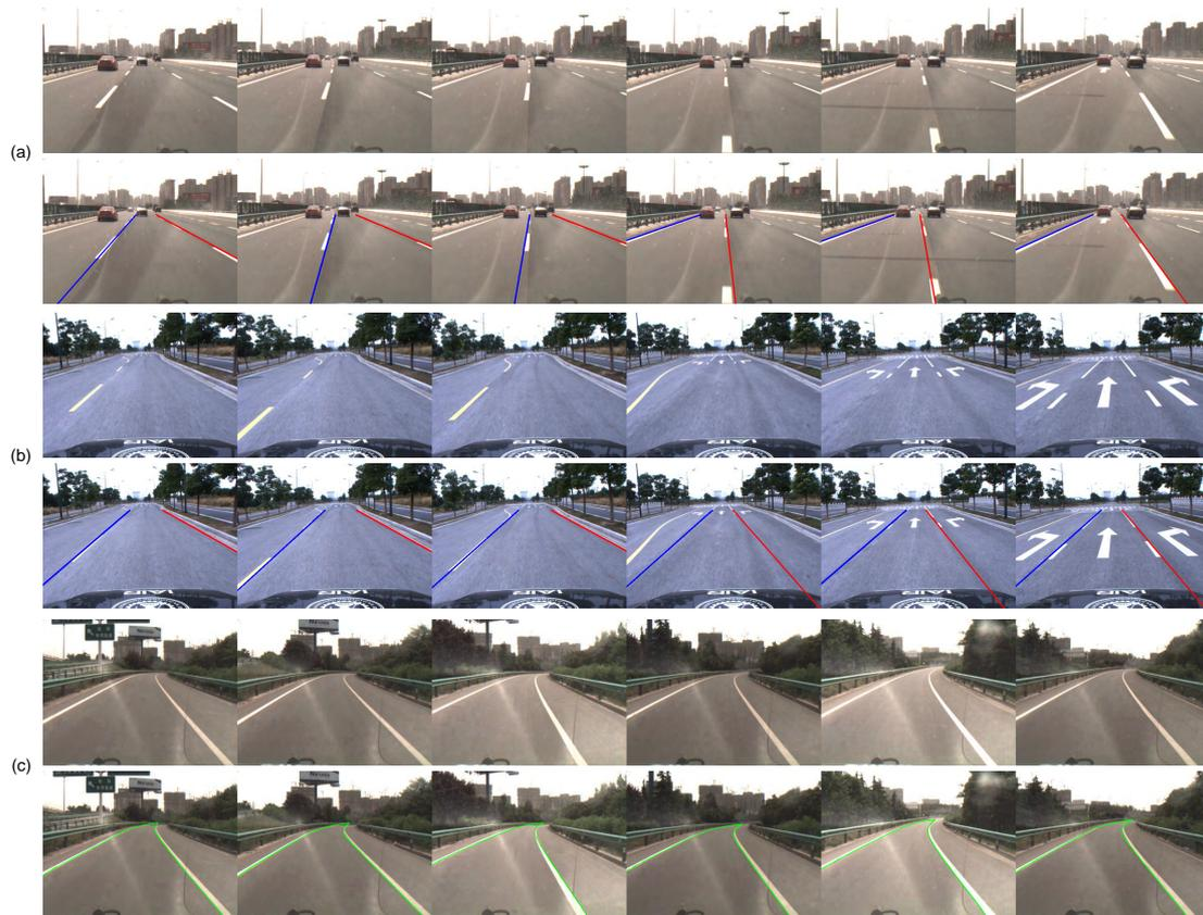
**Figure 12.** Examples of lane detection in road structure changes. (a) In the process of changing lanes; (b) Lanes suddenly become narrow; (c) Curved roads.
