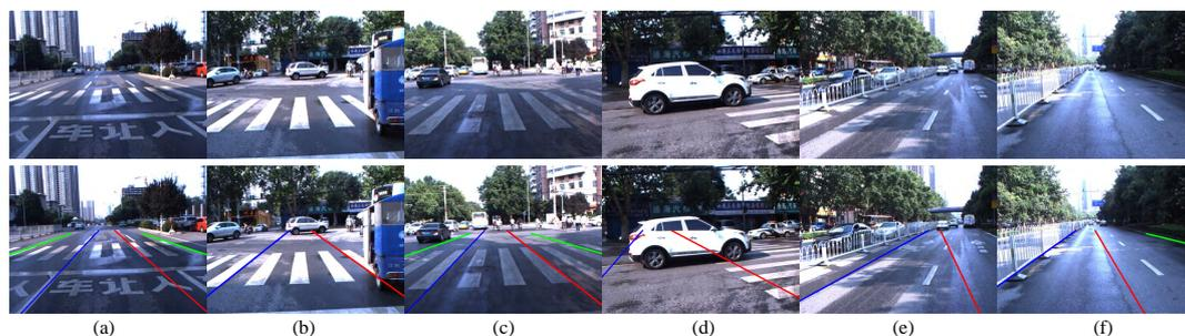
**Figure 14.** Examples of false positives. (a–c) Zebra crossings; (d,e) Crossroads; (f) Wet roads.
