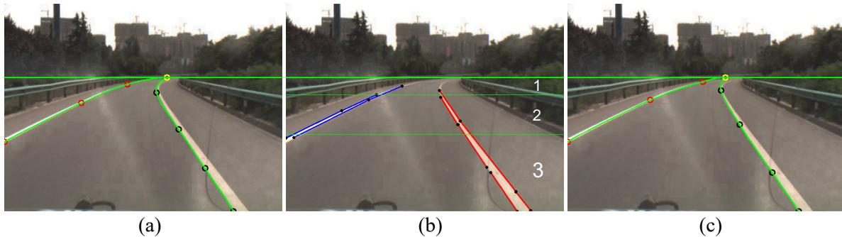
**Figure 9.** Curve lane boundary fitting. (a) Lane boundaries and control points in the  $n$ -th frame; (b) Computing the control points in the  $(n + 1)$ -th frame; (c) Lane boundaries and control points in the  $(n + 1)$ -th frame.
