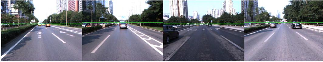
**Figure 3.** Examples of vanishing line detection.
