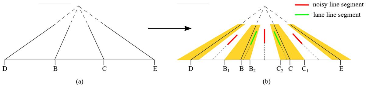
**Figure 6.** Illustration of the structure triangular filter. (a) The structure triangle; (b) Line segments filtering with the structure triangle; the yellow regions indicate the lane tolerance regions.
