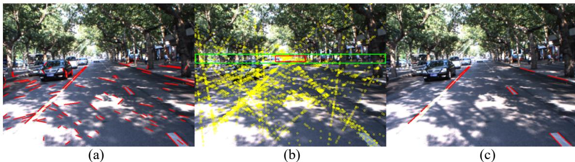
**Figure 4.** Illustration of the Crossing Point Filter (CPF). (a) Original feature map; (b) The vanishing box (red box) and the restrictive region (green box); the yellow points are the crossing points of all line segments; (c) The CPF result.
