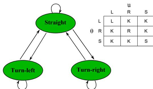
**Figure 7.** Road state machine. L, R, S and K denote ‘left’, ‘right’, ‘straight’ and ‘keep’, respectively.
