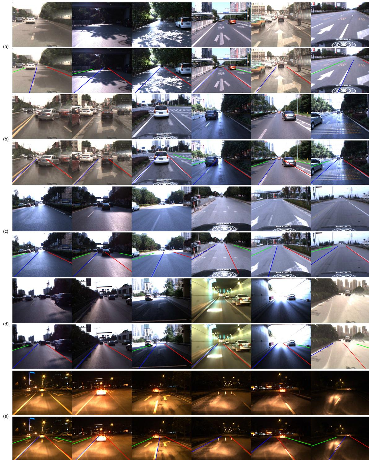
**Figure 11.** Examples of lane detection in various scenes. (a) Roads with shadows and paint; (b) Vehicle disturbance; (c) Worn lane boundaries; (d) Complex illumination; (e) Night.
