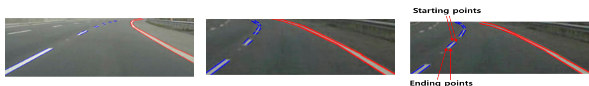
Figure 17. Examples of detection results on curve lanes of SLD datasets by our method (Detected dashed and solid lanes are shown in blue and red colors, respectively).
