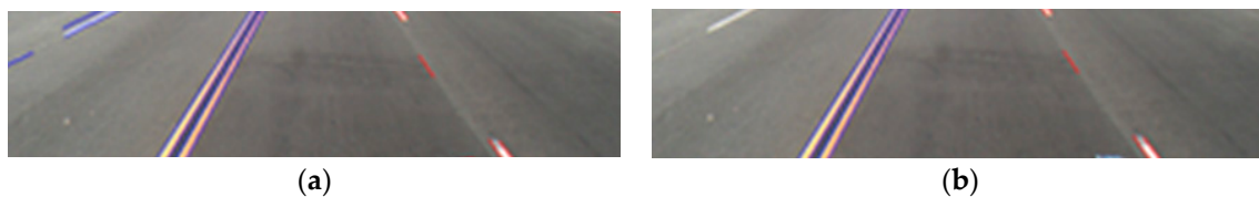
Figure 7. Removing the incorrect line segments based on angle features: (a) image including the detected line segments; and (b) image with the incorrect line segments removed.
