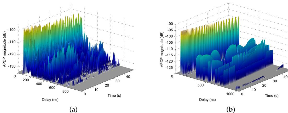
**Figure 3.** Evolution of averaged power delay profiles (APDPs) over time for TX position Tx1 and mobile RX on Track Rx1 from (a) measurement and (b) simulation.
