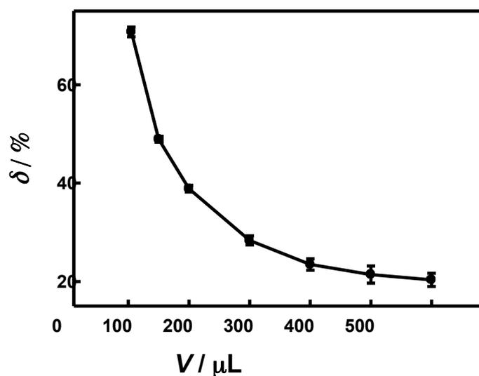
**Figure S1.**  $\delta$  versus volume of 0.1 M HNO<sub>3</sub> used to dissolve CdS QDs for our protocol ( $n = 3$ ). Conditions: 500-s enrichment; others are the same as in Figure 1 except for varying volume of HNO<sub>3</sub>.
