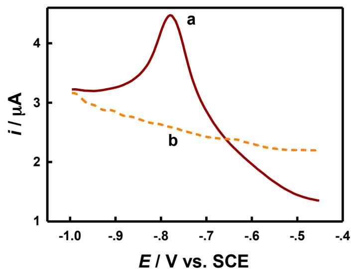
**Figure S2.** Differential pulse ASV responses at a BSA/anti-CEA/GA-CS/SPCE (a) and a neighboring bare SPCE (b). The electrodes were incubated with  $40 \text{ fg}\cdot\text{mL}^{-1}$  CEA and then  $\text{Ab}_2\text{-CdS}$  QDs, and the ASV analysis was then performed. Here, only the immunoelectrode showed an ASV peak, while no obvious response was observed at the bare SPCE.
