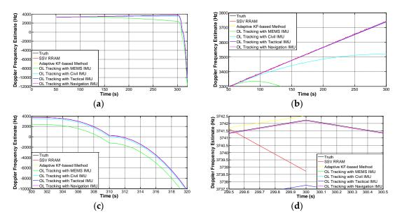
**Figure 9.** Comparison of the estimated Doppler frequency using different tracking schemes in the experiments. (**a**) Global view; (**b**) viewport of the second phase (non-maneuvering); (**c**) viewport of the third and fourth phase (maneuvering); and (**d**) close-up view around the 300th s.
