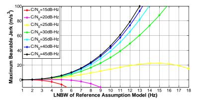
**Figure 2.** The maximum bearable LOS jerk under different  $C/N_0$  for SSV RRAM.
