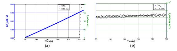
**Figure 6.** The variation of  $C/N_0$  and LOS jerk for the established scenario. (a) Global view; and (b) close-up view of the second phase.
