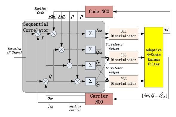
Figure 3. Block diagrams of adaptive four-state KF-based tracking strategy.
