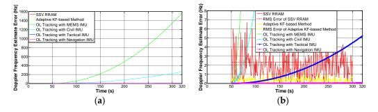
**Figure 10.** Comparison of Doppler estimation errors using different tracking schemes in the experiments. (a) Global view; and (b) close-up view.
