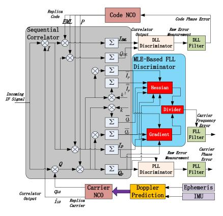
Figure 4. Suggested architecture of INS-assisted open loop tracking.
