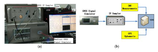
**Figure 7.** The distribution and connection of the instruments in the experiment. (**a**) Physical connection; and (**b**) schematic connection.
