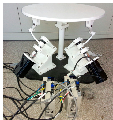
Figure 19. Field photo of the 2-DOF SPM prototype.
