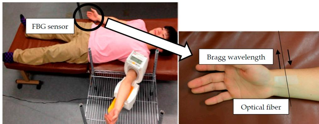
**Figure 3.** Experimental image of blood pressure measurement by the FBG sensor.
