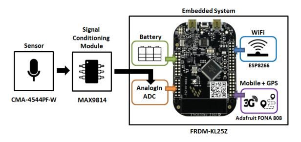
**Figure 1.** Suggested hardware platform. This is based on the FRDM-KL25Z embedded system. The microphone is the CMA-4544PF-W capsule followed by the MAX9814 amplifier. The platform also provides GPS, WiFi and mobile communications modules.
