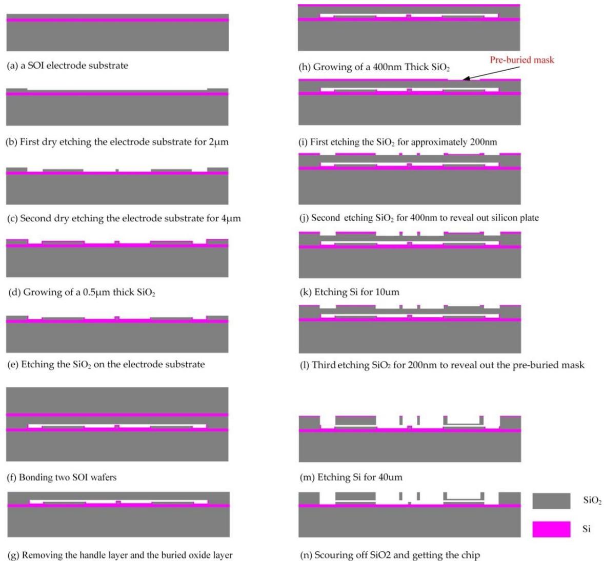
**Figure 12.** The fabrication process of the accelerometer.
