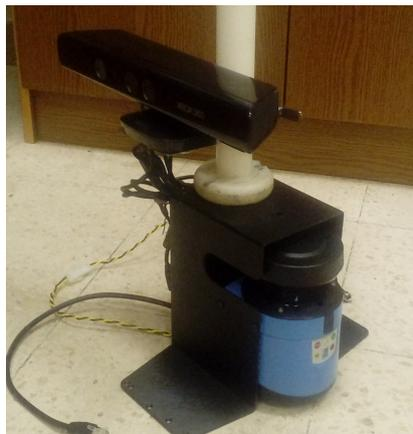
**Figure 17.** A configuration where the views of the sensors are in different planes.
