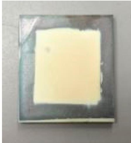
**Figure 1.** Optical image of 50- $\mu$ m-thick and 400 mm<sup>2</sup> Mn-doped CBT/PZT films fabricated on 3-mm-thick and 900 mm<sup>2</sup> titanium substrate.
