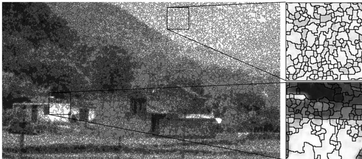
**Figure 3.** The segmentation result with watershed algorithm on an ICCD image.
