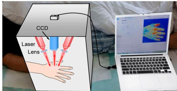
**Figure 1.** Portable imaging box developed for the imaging data acquisition.
