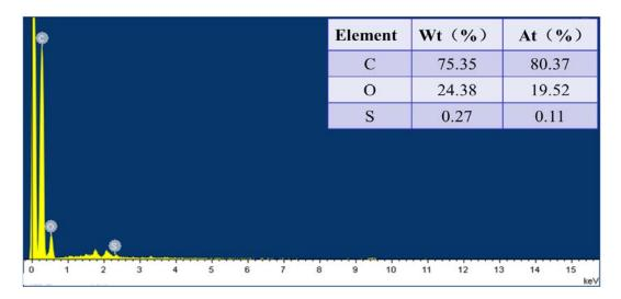
**Figure 2.** The energy-dispersive X-ray spectroscopy (EDX) spectra of sulfophenyl-functionalized reduced graphene oxide (SFRGO).
