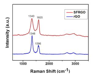
Figure 4. Raman spectra of SFRGO and reduced graphene oxide (rGO).
