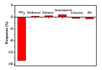
**Figure 6.** Gas sensing selectivity of the SFRGO network film devices to 10 ppm NO<sub>2</sub> and 25 ppm methanol, 25 ppm ethanol, 25 ppm chlorine, and 50% relative humidity.
