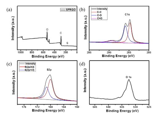
**Figure 3.** (**a**) The X-ray photoelectron spectroscopy (XPS) spectra of SFRGO. XPS spectra for (**b**) C 1s, (**c**) S2p, and (**d**) O 1s.
