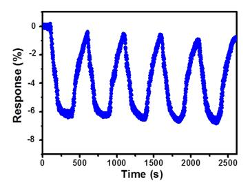
Figure 7. The sensing repeatability for the SFRGO network film devices to 500 ppb NO<sub>2</sub>.
