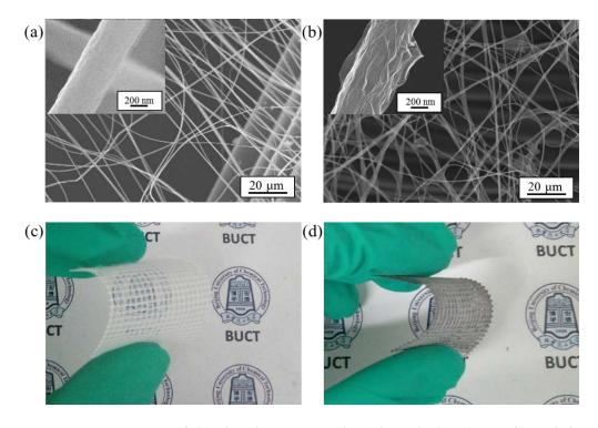
**Figure 1.** SEM images of (**a**) the electrospun polyacrylonitrile (PAN) nanofiber skeleton (inset: the high-resolution SEM image), (**b**) the wrapped SFRGO onto the PAN nanofiber skeleton (inset: the high-resolution SEM image). Photographs of (**c**) the electrospun PAN nanofibers on the nylon scaffold, and (**d**) the flexible SFRGO network films. The school badges are placed behind the film.
