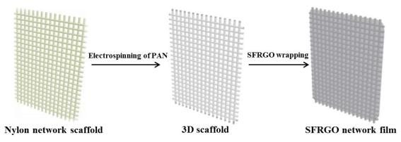
**Scheme 1.** Schematic illustration for the fabrication of the sulfophenyl-functionalized reduced graphene oxide (SFRGO) network films by assembling the SFRGO onto an electrospun 3D nanonetwork skeleton.
