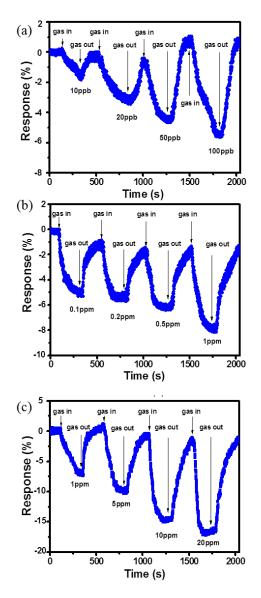
**Figure 5.** Sensing performance of the SFRGO network film devices to different concentrations of NO<sub>2</sub>, from 10 ppb to 20 ppm ((**a**) 10–100 ppb; (**b**) 100–1000 ppb; (**c**) 1 ppm–20 ppm).
