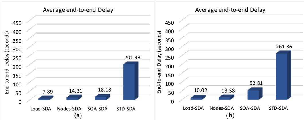
**Figure 22.** Average end-to-end delay for the monitoring traffic with a shorter beacon interval: (a) Unconditioned Scenario; (b) Conditioned Scenario.
