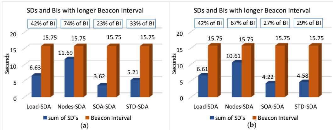
**Figure 18.** Beacon Interval and average sum of superframe durations for a network with a longer beacon interval in the: (a) Unconditioned Scenario; (b) Conditioned Scenario.
