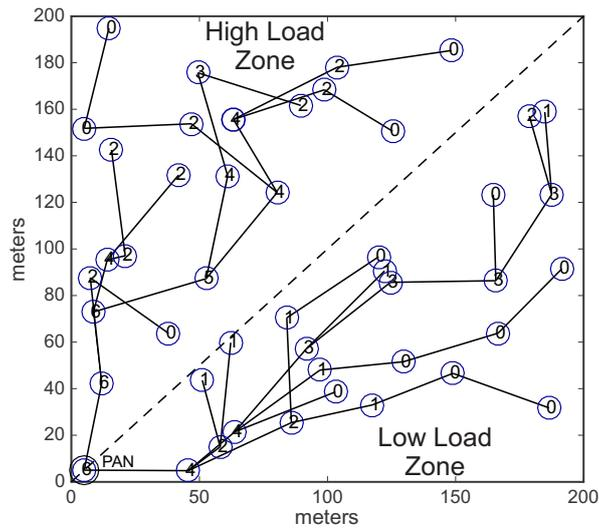
**Figure 24.** An example of Superframe Order configuration for all cluster-heads, using Load-SDA scheme (conditioned Scenario).
