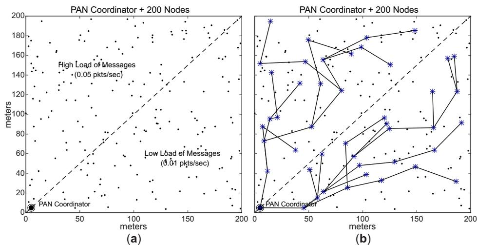
**Figure 13.** Configuration of the *conditioned Scenario*: (a) Data rates distributed in two load zones; (b) Conditioned cluster-tree network.
