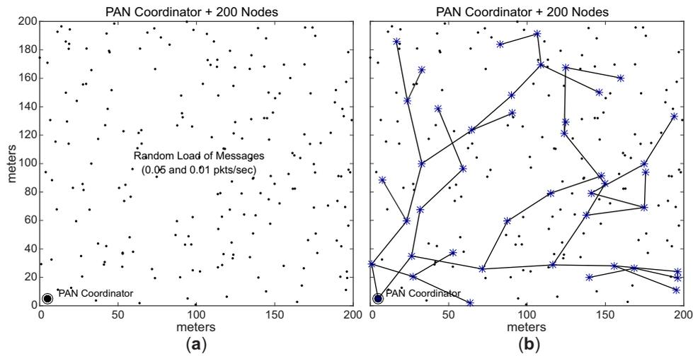
**Figure 12.** Configuration of the *unconditioned Scenario*: (a) Randomly distributed data rates; (b) Unconditioned cluster-tree network.
