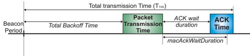
**Figure 8.** Transmission time duration of a data frame.
