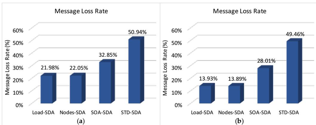
**Figure 17.** Message loss rate for the SDA schemes: (a) Unconditioned Scenario; (b) Conditioned Scenario.
