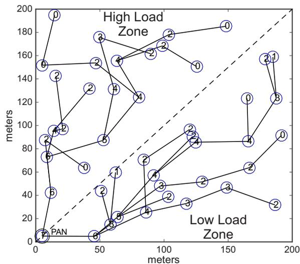
**Figure 25.** An example of Superframe Order configuration for all cluster-heads, using Nodes-SDA scheme (conditioned Scenario).
