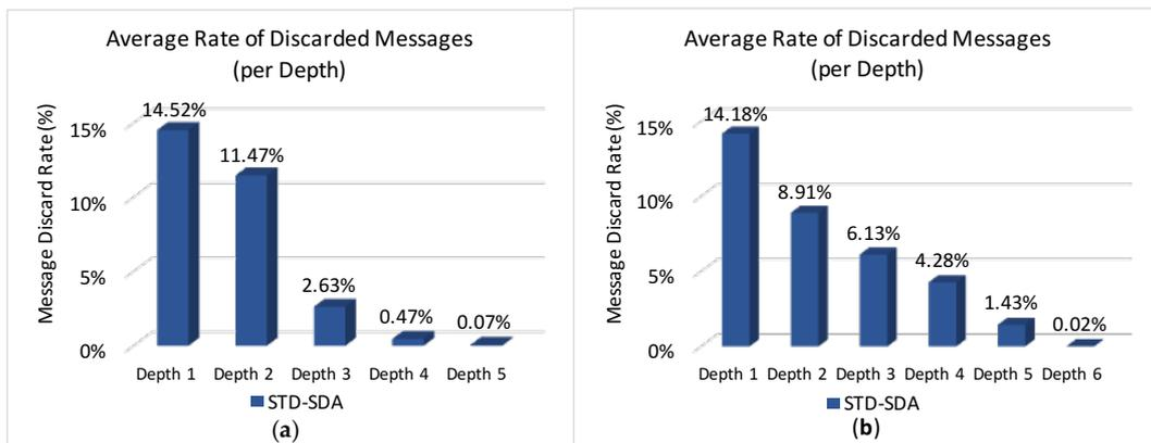
**Figure 15.** Average message discard rate (per depth) due to buffer overflows for the STD-SDA scheme: (a) Unconditioned Scenario; (b) Conditioned Scenario.
