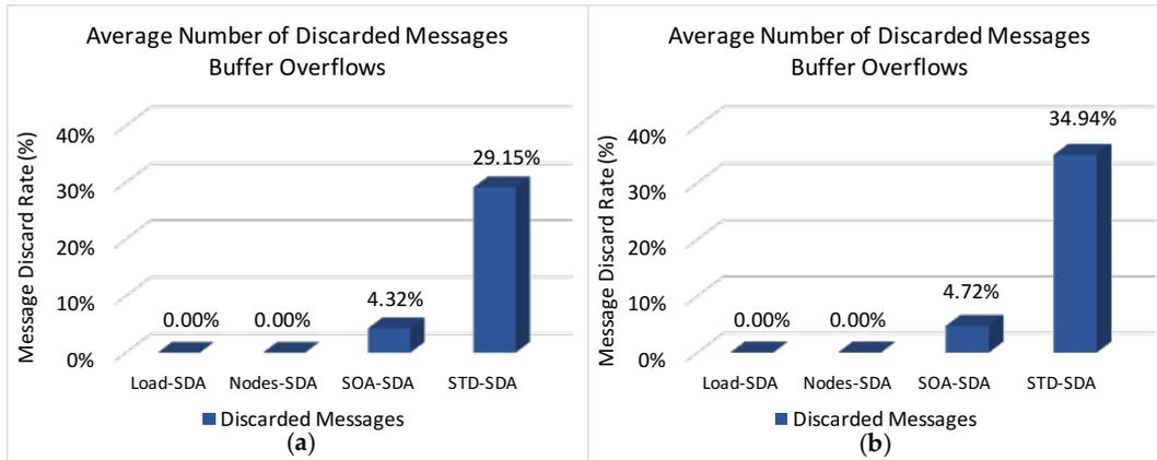
**Figure 14.** Average discard message rate due to buffer overflows: (a) Unconditioned Scenario; (b) Conditioned Scenario.
