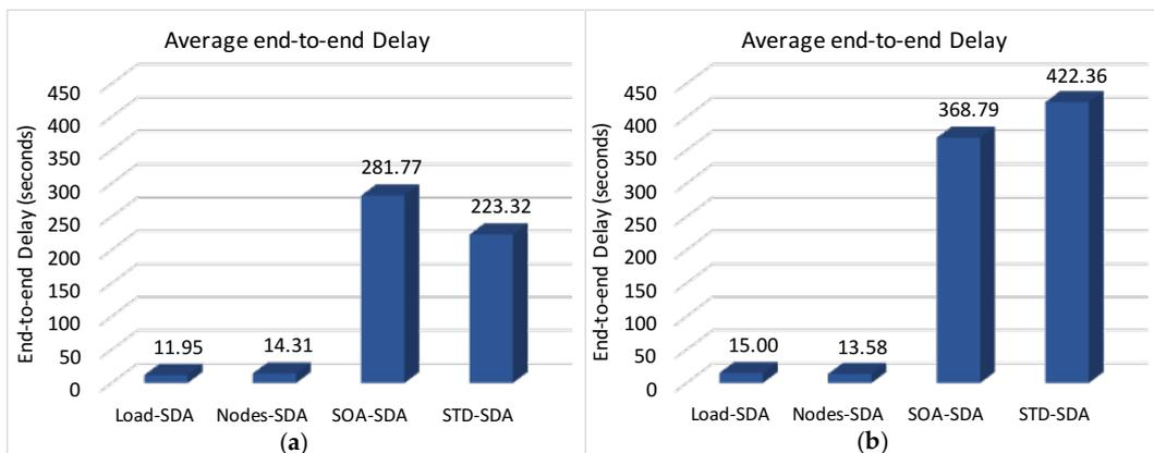
**Figure 19.** Average end-to-end communication delay for a network with a longer Beacon Interval in the: (a) Unconditioned Scenario; (b) Conditioned Scenario.
