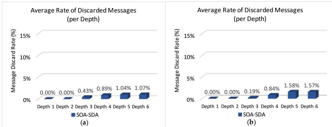
**Figure 16.** Average message discard rate (per depth) due to buffer overflows for the SOA-SDA scheme: (a) Unconditioned Scenario; (b) Conditioned Scenario.
