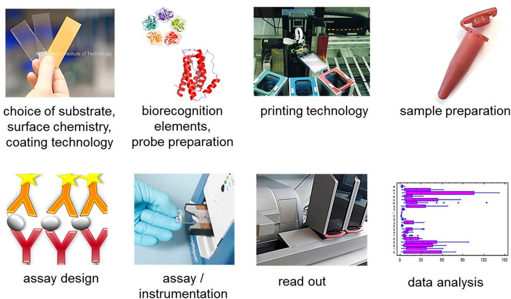
**Figure 1.** Components of protein microarray production and processing. Work flow from left to right: Preparation of the immobilization surface, probe preparation, printing, sample preparation, assay design, instrumentation, read-out and data analysis.
