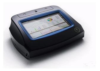
Figure 3. Photo of the QCM-based e-nose.
