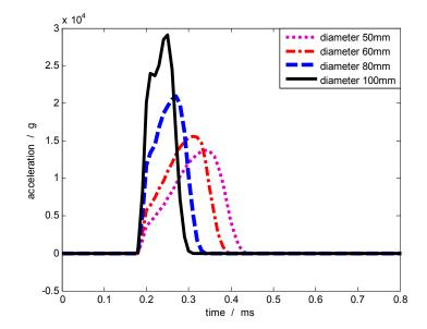
Figure 9. Acceleration pulse waveforms generated by different contact areas.
