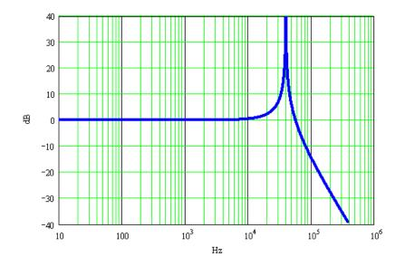
Figure 2. Amplitude-frequency characteristics of the accelerometer.
