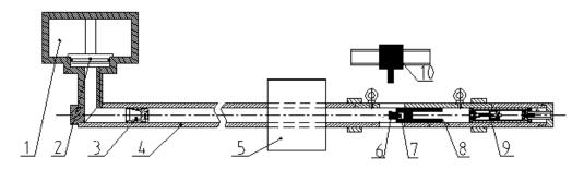
**Figure 5.** Schematic diagram of the quasi-static calibration system. (1) High-pressure gas chamber; (2) valve; (3) projectile; (4) launching tube; (5) silencer; (6) collision object (sensor mounting base); (7) calibrated accelerometer; (8) guiding cylinder; (9) liquid gas buffer device; and (10) laser interferometer.
