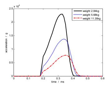
**Figure 8.** Acceleration pulse generated at the same projectile velocity but with different masses of the impacted body (diameter of the contact surface: 50 mm).
