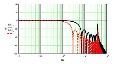
Figure 3. Sensor's frequency domain response to the two pulsed excitations.
