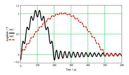
Figure 4. Sensor's time domain response to the two pulsed excitations.
