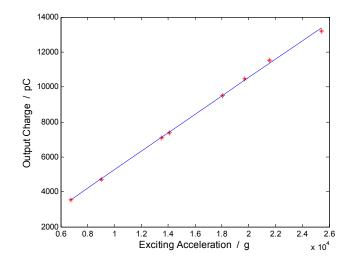
Figure 13. Fitted sensitivity curve of the calibrated accelerometer.
