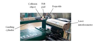
Figure 6. Photo of the projectile before collision with the collision object.
