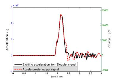
Figure 12. Excitation acceleration from laser interferometer and response acceleration from the accelerometer.
