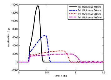
Figure 10. Acceleration pulse curves corresponding to different pad thicknesses.
