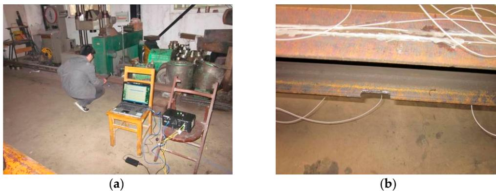
**Figure 12.** The steel beam experiment field: (a) dynamic test and data logger; and (b) damage simulation.
