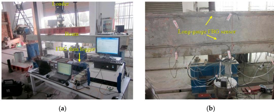
**Figure 19.** Experiment field: (a) beam specimen, loader and data logger; and (b) long-gauge FBG sensors.
