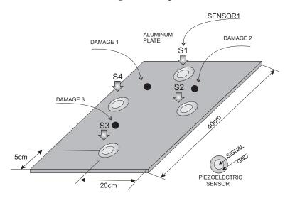
Figure 23. Aluminum plate instrumented with four piezoelectric sensors.
