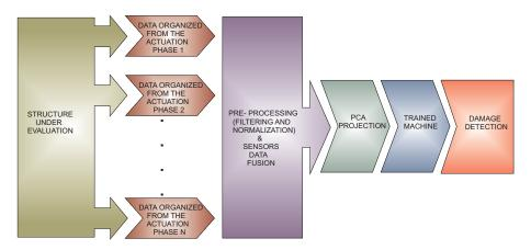
Figure 9. Testing step with data from the structure in an unknown structural state.
