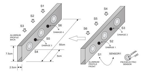
Figure 12. Aluminum rectangular profile instrumented with six piezoelectric sensors.
