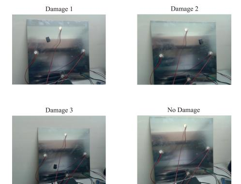
**Figure 24.** Experimental setup for the aluminum plate instrumented with four piezoelectric sensors and with different kind of damage.
