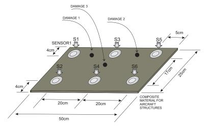
Figure 29. Composite plate instrumented with six piezoelectric sensors.
