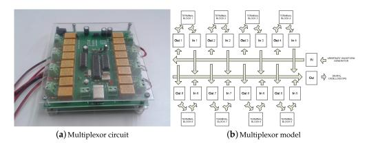
**Figure 5.** Multiplexor system used in the data acquisition system.
