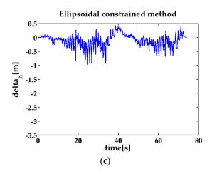
**Figure 5.** Left and right feet altitude difference in 2D the closed path experiment. (**a**) the height difference of the two feet without contraint; (**b**) the height difference of the two feet with spherical constraint; (**c**) the height difference of the two feet with ellipsoidal constraint.
