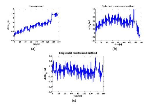
**Figure 7.** The left and right feet position altitude difference in the upstairs experiment. (**a**) the height difference of the two feet without constraint; (**b**) the height difference of the two feet with spherical constraint; (**c**) the height difference of the two feet with ellipsoidal constraint.
