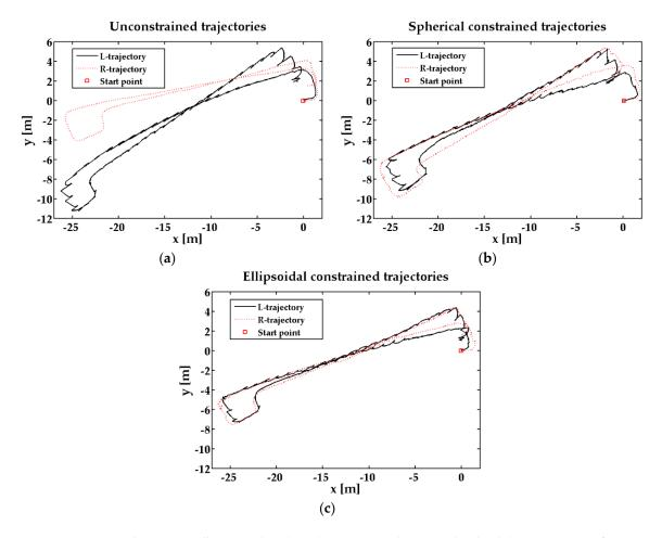
**Figure 4.** Pedestrian walking a closed path in a corridor outside the laboratory. (**a**) feet trajectories without constraint; (**b**) feet trajectories with spherical constraint; (**c**) feet trajectories with ellipsoidal constraint.
