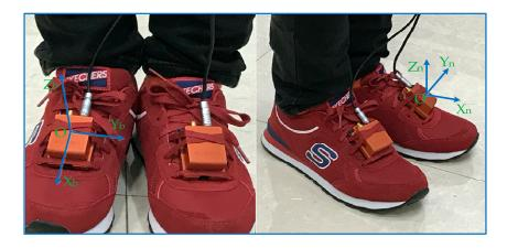
**Figure 1.** (Left) The two MIMU are mounted to the feet separately, the  $OX_bY_bZ_b$  coordinate system are the carrier coordinates; (right) side view, the  $OX_nY_nZ_n$  coordinate system are the navigation coordinates.
