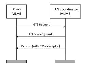
Figure 8. Assignment of GTS to the sensor node.
