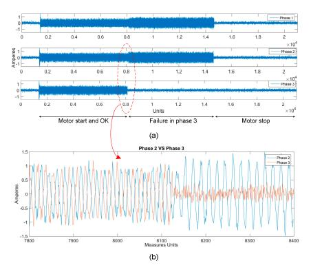
**Figure 19.** Detection of a fault in a phase by the current sensors. (**a**) Measured current for the three phases; (**b**) Zoom of the currents of the phases 2 and 3 in the area where the phase 3 fails.
