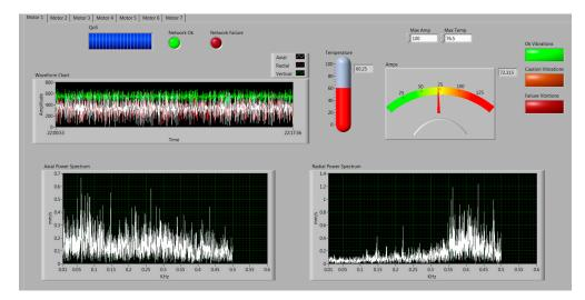
Figure 12. GUI designed for the monitoring application.
