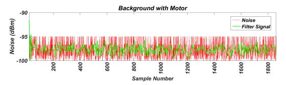
Figure 14. Measured background noise with motors running.
