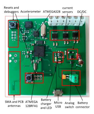
Figure 3. Photograph of the wireless sensor node.
