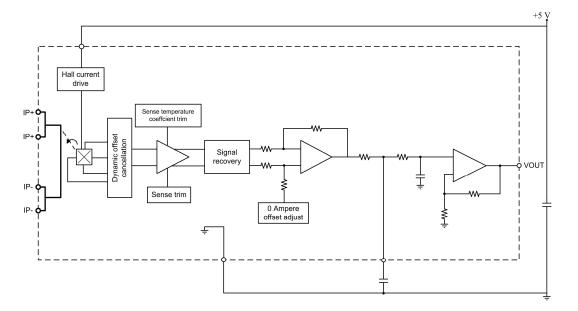
Figure 4. Functional block diagram of the current transducer.
