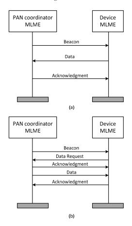
**Figure 9.** (**a**) Communication from the sensor nodes towards the coordinator node; (**b**) Communication from the coordinator node towards the sensing nodes.
