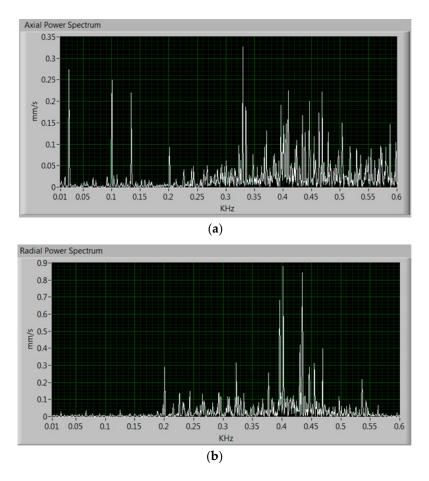
**Figure 17.** Measured power spectrum of the vibrations when the motor is running properly. (**a**) Axial vibrations and (**b**) radial vibrations.
