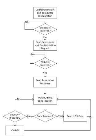
Figure 10. Flow chart of the coordinator node.
