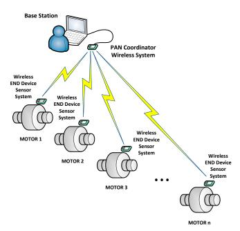
Figure 1. Architecture of the designed wireless sensor network.
