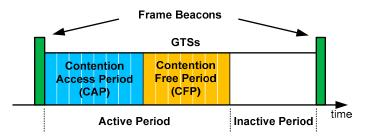
Figure 7. Beacon-enabled mode: superframe structure with GTSs.
