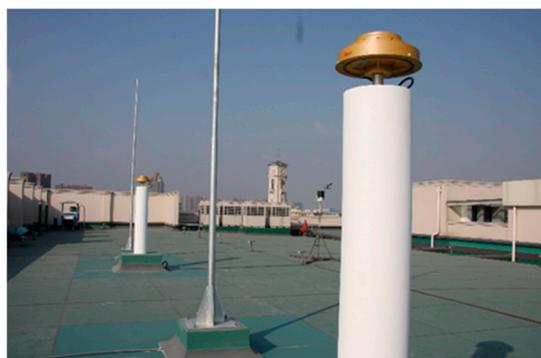
**Figure 3.** GNSS reference stations in UNNC.
