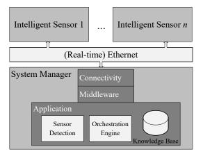
Figure 2. Architecture of the fusion system [52].
