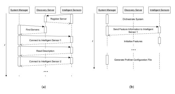
**Figure 4.** Communication sequences between system manager, discovery server, and intelligent sensors for SEFU/IFU system configuration. (a) Sequence describing the detection of intelligent sensors [52]; (b) Communication of feature information for assigning feature computation tasks to intelligent sensors.
