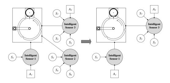
Figure 7. Rejection of one intelligent sensor from the fusion system architecture.
