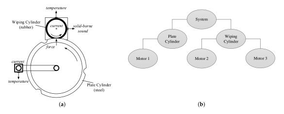
**Figure 6.** Set-up of the printing unit demonstrator. (a) Structural design of the printing unit demonstrator [6]; (b) Hierarchy of the demonstrator [7].
