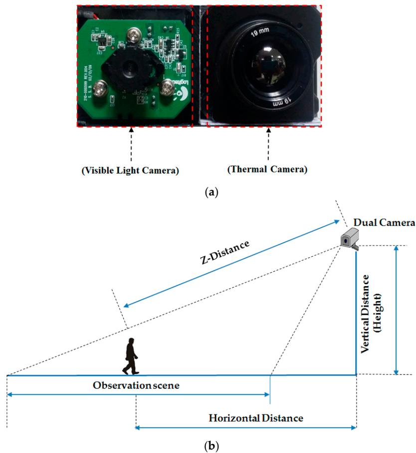
**Figure 6.** Dual visible light and thermal camera and experimental setup for data acquisition in our study: (a) the dual visible light and thermal camera; and (b) the experimental setup.
