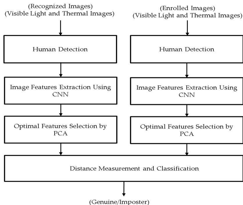
Figure 1. Overall procedure of proposed method for person recognition.
