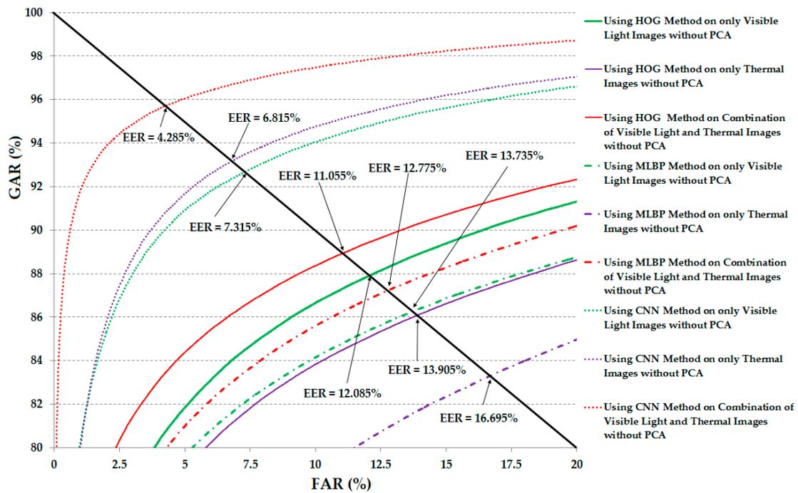
**Figure 10.** Receiver operating curves (ROC) of the verification systems (system that uses only visible light, only thermal, and a combination of visible light and thermal images for verification) using Euclidean distance without applying principal component analysis (PCA).
