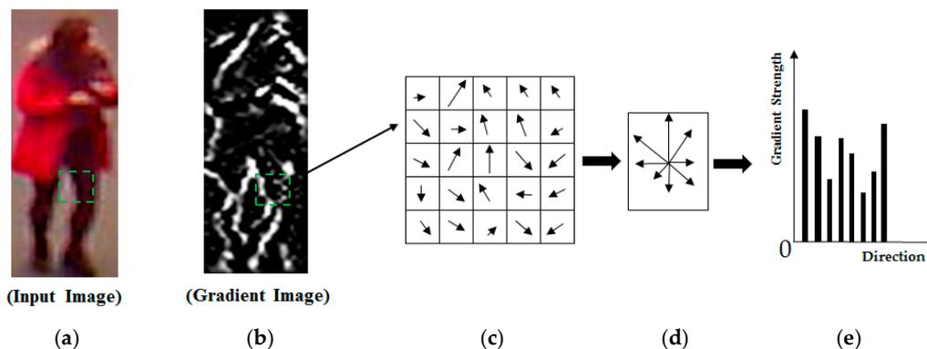
**Figure 2.** Methodology of image features extraction using the histogram of oriented gradients (HOG) method: (a) input image with a given sub-block; (b) the gradient image of (a); (c) the gradient map of the green sub-block in (a,b); (d) the accumulated strength and direction information of the gradient at every pixel in the green sub-block; and (e) the final extracted feature for the green sub-block.
