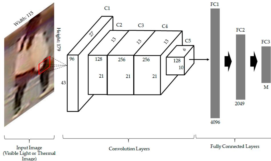
**Figure 5.** The designed convolutional neural network (CNN) structure for person recognition in our proposed method.
