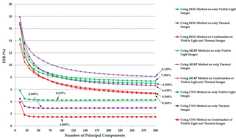
**Figure 14.** Verification accuracy (EER) of the recognition systems using correlation distance according to the number of principal components in PCA.
