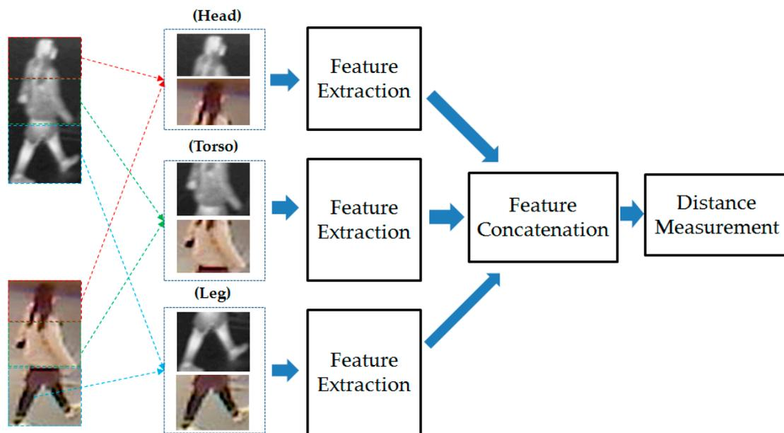
**Figure 20.** Flowchart of gender recognition using the combination of different body parts.
