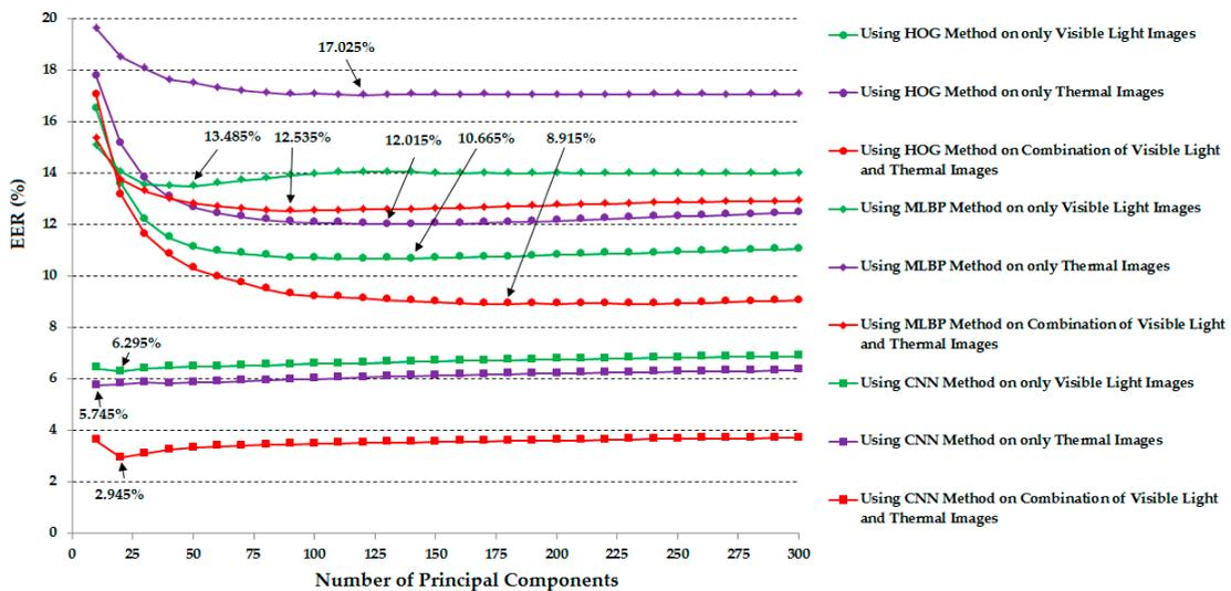
**Figure 11.** Verification accuracy (EER) of the recognition systems using Euclidean distance according to the number of principal components in PCA.
