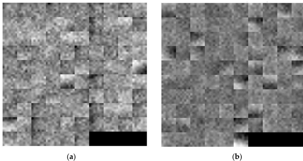
**Figure 9.** The 96 trained convolution filters in the size of  $7 \times 7 \times 1$  obtained in the first convolution layer using our CNN configuration in Figure 5 and our training database: (a) the filters obtained using visible light images, and (b) the filters obtained using thermal images.
