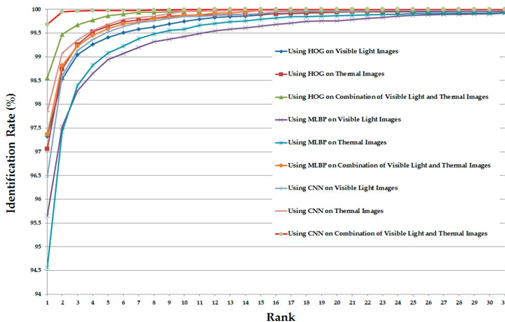
**Figure 12.** Cumulative matching characteristic curve (CMC) curves using Euclidean distance with various system configurations for the identification problem.
