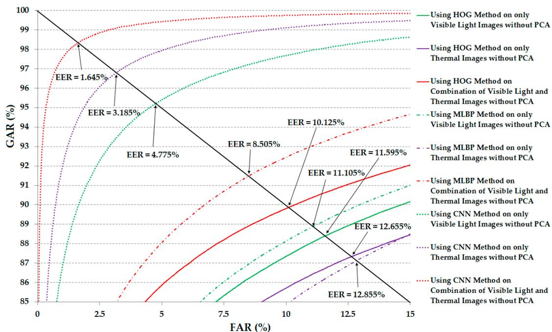
**Figure 13.** ROC curves of the verification systems (system that uses only visible light, only thermal, and a combination of visible light and thermal images for verification) using correlation distance without applying PCA.
