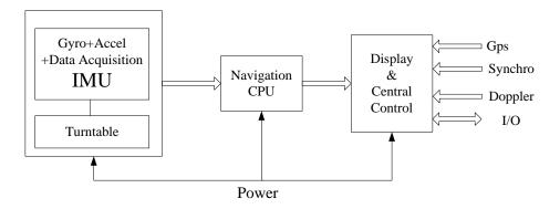
Figure 6. A functional diagram of the designed dual-axis rotational INS.
