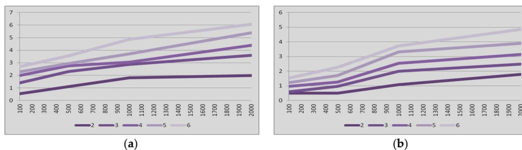
**Figure 5.** Latency (vertical, seconds) vs. inactivity interval (horizontal, milliseconds). Links always in *park* mode. From two to six hops: (a) *master-to-slave* communication; (b) *slave-to-master* communication.
