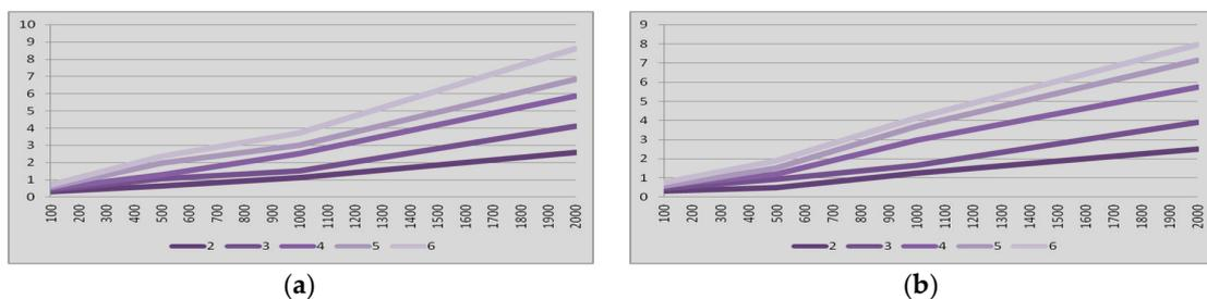
**Figure 7.** Latency (vertical, seconds) vs. inactivity interval (horizontal, milliseconds). Links always in *sniff* mode. From two to six hops. (a) *master-to-slave* communication; (b) *slave-to-master* communication.
