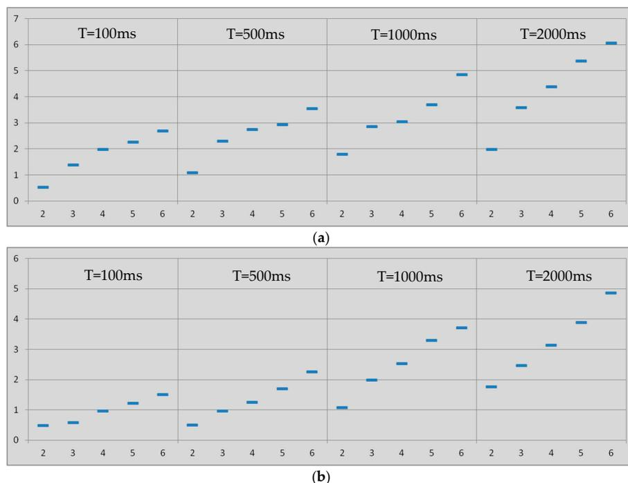
**Figure 4.** Latency (vertical, seconds) vs. amount of hops (horizontal). Links always in *park* mode. Inactivity intervals (from left to the right): 100, 500, 1000 and 2000 ms. (a) *master-to-slave* communication; (b) *slave-to-master* communication.
