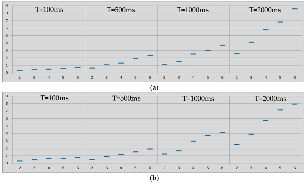
**Figure 6.** Latency (vertical, seconds) vs. amount of hops (horizontal). Links always in *sniff* mode. Inactivity intervals: 100, 500, 1000 and 2000 ms. (a) *master-to-slave* communication; (b) *slave-to-master* communication.
